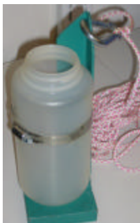
Figure 2.7 Bridge sampler with high density polypropylene nalgene bottle.
