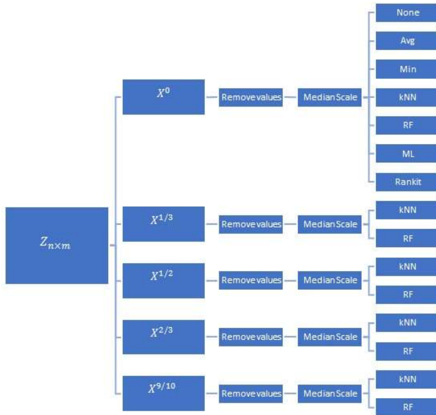
Figure 2.14.16: Feature set simulation workflow. Each experiment comprises 1,000 simulations. Z_{n \times m} is a multivariate standard normal from which X^p is constructed with pairwise (spearman) correlation \rho for all vectors. Normal simulations involve X^p being multivariate normal while the non-normal simulations consist of log-normal and uniform. In all cases, values removed are done so by taking the lowest from the variables selected. For the normal simulation case, simulations are also performed by removing values at random.
