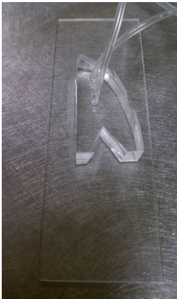
Figure 5.2: “V” Shape Collection System
