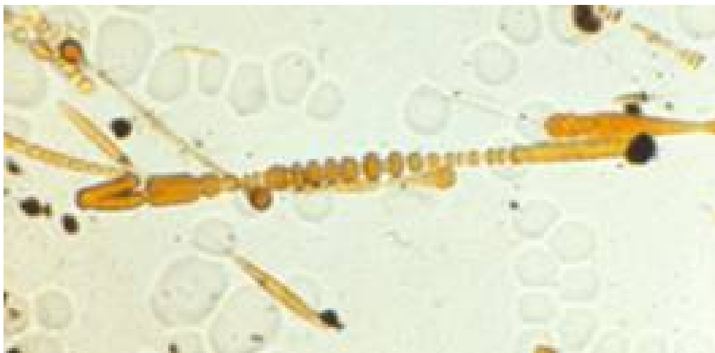
Figure 1.5. Scanning Electron microscope image of asbestos fiber with ferruginous bodies associated with its surface at a magnification of 2,000.
