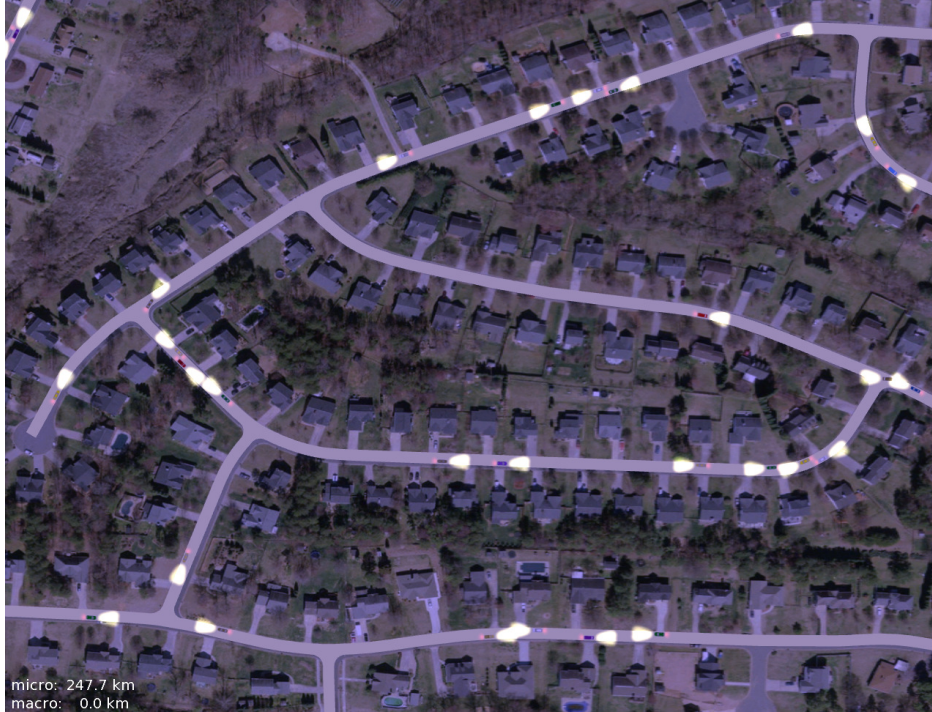
Figure 2.1: A road network generated directly from GIS data by my method. The road network has been overlaid on top of a satellite image. Note that the cars on the road network are animated using a traffic simulator running on my road network representation.
