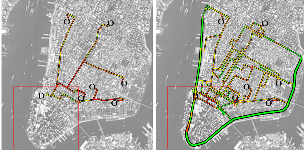
Figure 5.6: An example of the MSSD scenario: in which vehicles are spawned at various origin points and drive to a single destination. On the left is the mean velocity field of the fastest-path baseline router, and on the right is the mean velocity field resulting from my method. The destination point was chosen randomly inside the destination region, designated by the red rectangle. The origin points were chosen randomly outside this region with the additional constraint that they be at least 1km away from the destination. The mean velocity is shown as a color ranging from red, 0 m/s, to green, 13 m/s, the speed limit for most of the roads.
