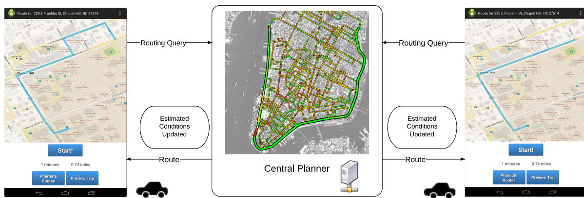
Figure 5.1: A System Architecture of Participatory Route Planning: The mobile clients send route queries to the central planner, which takes the updated traffic and routing information from participants and live traffic sensor information to plan a new route for each participating client in the network.
