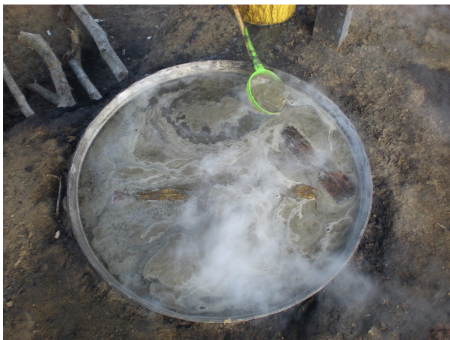
Figure 64. Panela production #3: Boiling the cane juice into syrup. Notice the wood pieces added for additional nutrients and flavor, with a community member removing the film that concentrates at the surface. Source: Author photo.
