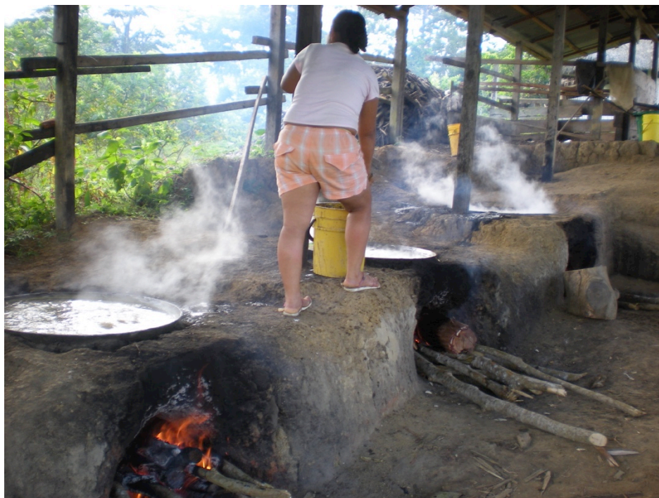
Figure 65. Panela production #4: Community member tending to multiple pots of boiling cane juice. Source: Author photo.
