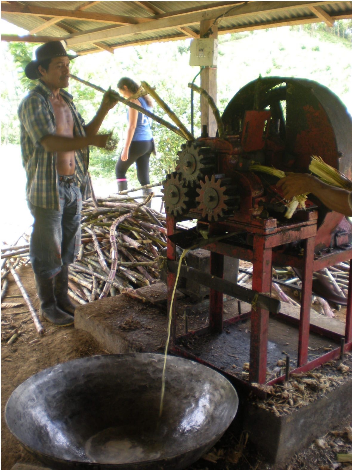
Figure 62. Panela production #1: Extracting juice from the cane stalks. Source: Author photo.
