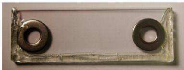
Figure A.3: Homemade cuvette used to contain dye-sensitized films during transient absorption experiments.
