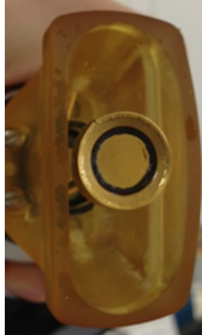
Figure 3.1: This photograph shows the center high frequency element (25 MHz) surrounded by the low frequency annular element (4MHz). Both elements have curved lenses to focus them to a depth of 15 mm.
