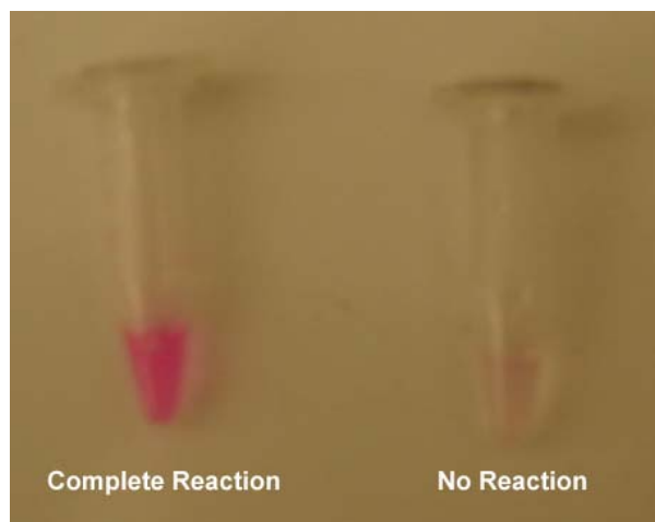
Figure 4.3. The resorufin ADP/ P_i reporter molecule provides a convenient colorimetric indicator that the reaction is complete. On the left, a complete positive control reaction is dark pink at the end of the experiment, while on the right, a negative control reaction is essentially colourless.
