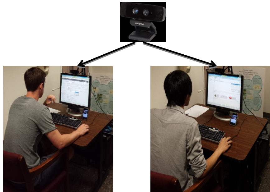
Figure 4.3: Experimental setup that shows placement of the Creative® Interactive Gesture Camera.
