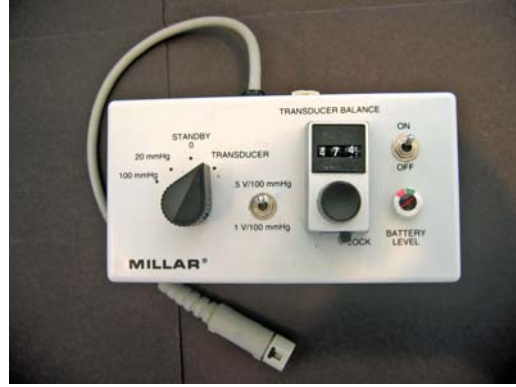
Figure 2.1 Photographs of a Millar™ Mikro-Tip intravascular A) pressure transducer catheter and B) control box.
