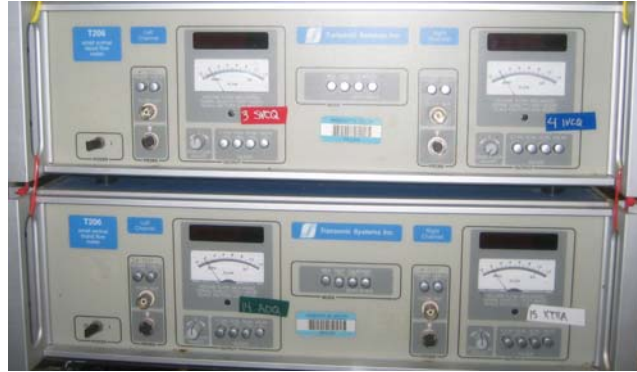
Figure 2.2 Photographs of A) Transonic™ transit-time flow probe and B) Transonic™ T206 small animal flow control unit.
