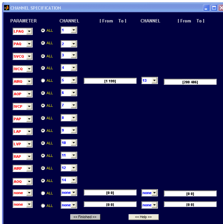
Figure 2.11 Channel specification GUI developed for channel number array creation. An example using multiple channels for airway flow (AIRQ) is illustrated. Pull-down menus allow for hemodynamic variable and channel number selection. Text boxes create array indices.
