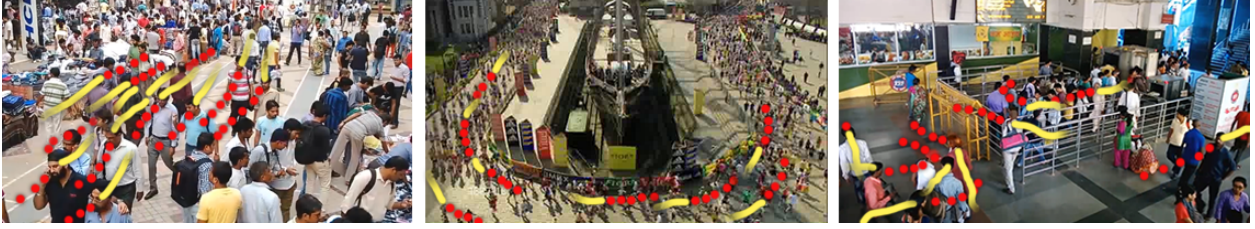
Figure 3.3: Prediction Outputs We test our approach on a variety of crowd datasets with varying density. Our approach had a benefit of upto 18% better prediction at a 5 second time horizon for some high-density datasets. Yellow lines represent past tracked trajectories whereas the red dots represent predicted motion.
