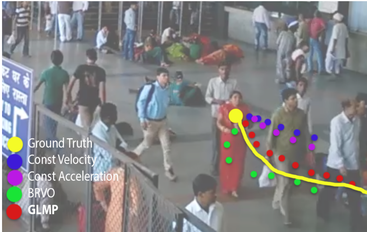
Figure 3.1: Improved Prediction We demonstrate the improved accuracy of our pedestrian path prediction algorithm (GLMP) over prior real-time prediction algorithms (BRVO, Const Vel, Const Accel) and compare them with the ground truth. We observe upto 18% improvement in accuracy.
