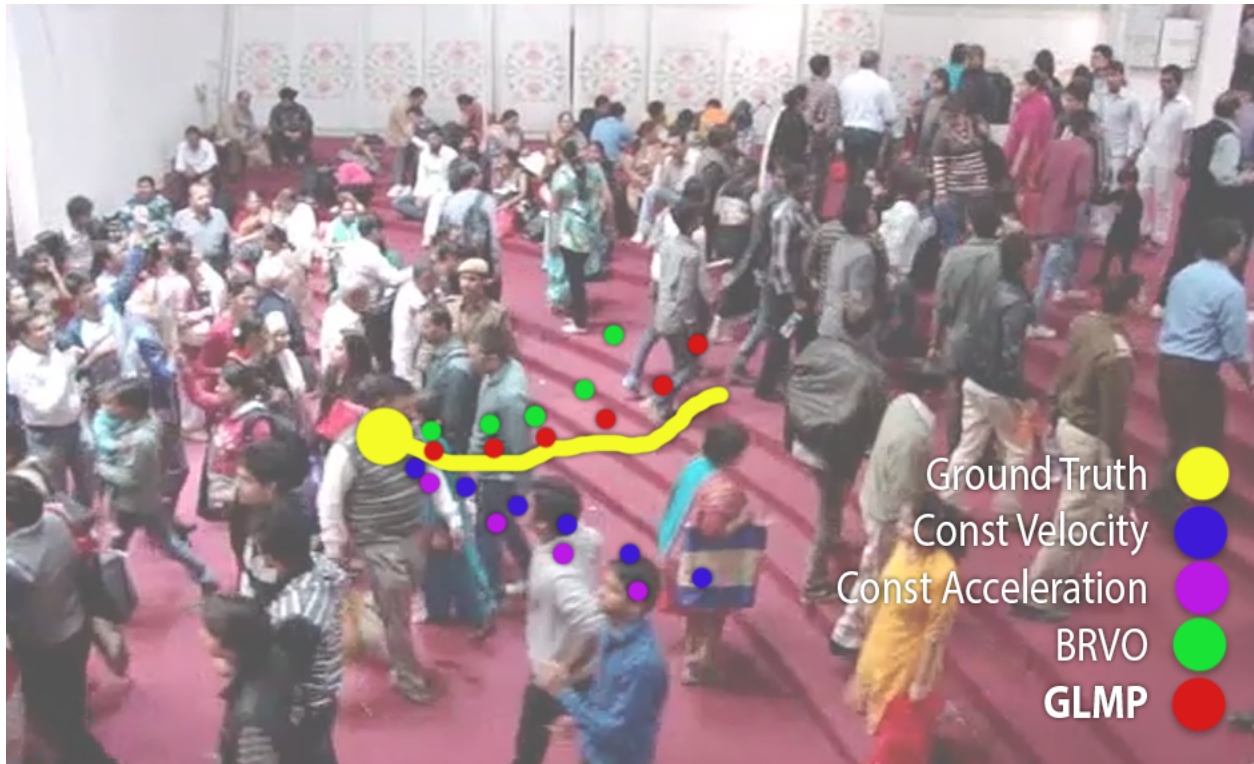
Figure 3.5: Improved Prediction We demonstrate the improved accuracy of our pedestrian path prediction algorithm (GLMP) over prior real-time prediction algorithms (BRVO, Const Vel, Const Accel).
