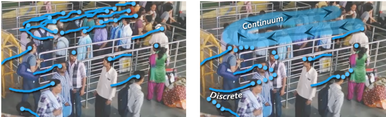
Figure 2.2: The left image highlights the tracked trajectories based on discrete motion models. The image on the right demonstrates the use of a hybrid motion model, using the continuum method for a cluster of pedestrians as well as discrete motion models for individuals. These clusters are computed in realtime based on frame coherence and pedestrian flow. The hybrid motion model can improve the tracking accuracy in these dense scenarios by 20% over prior methods.
