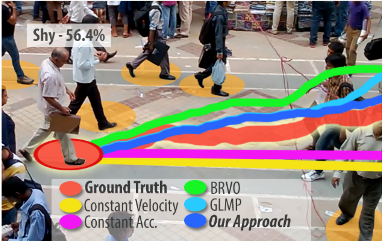
Figure 5.12: Our approach automatically classifies pedestrian behaviors in real-time (e.g. Shy behavior of a pedestrian). This behavior information is used to dynamically compute motion parameters and improve the performance of our long-term prediction algorithm (shown in dark blue) and compute proxemic distances. Our results are very close to ground truth (shown in red) and offer up to 21% improvement over prior real-time algorithms, whose predicted trajectories are shown in different colors. This demonstrates the benefits of using the psychological constraints for prediction and navigation.
