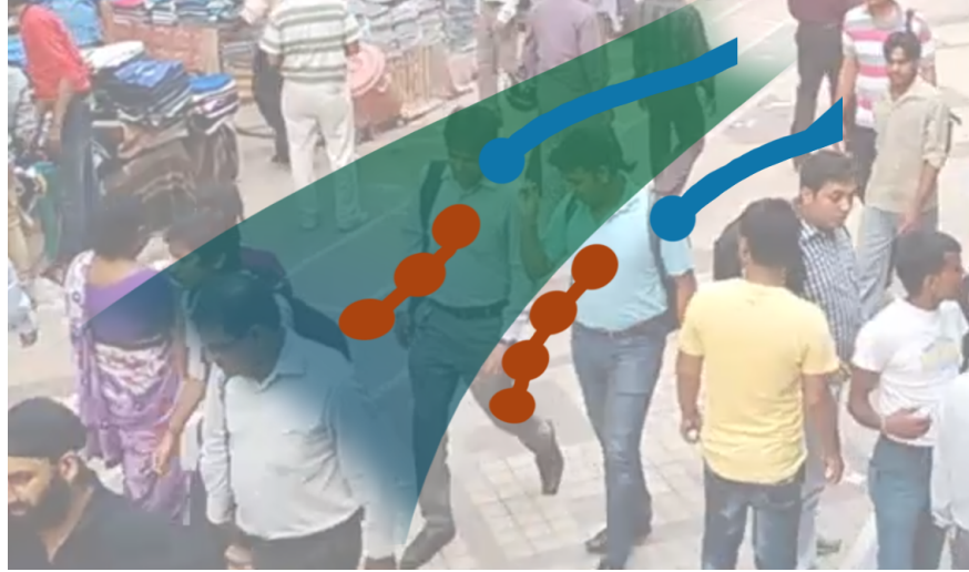
Figure 3.4: Global vs Local Movement Patterns The blue trajectories indicate prior tracked data. The red dots indicate local predicted patterns retrieved from learning macro and microscopic simulation models, The shaded (green-blue) path represent the global movement patterns learned from the path data in that cluster
