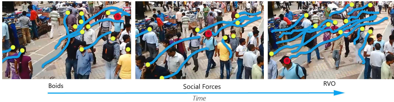
Figure 2.3: Our microscopic mixture motion model can accurately compute the trajectories in real time. We highlight different motion models (Boids, Social-Forces, or reciprocal velocity obstacles) used for the same pedestrian (marked in red) over different frames. We believe that it is not possible to model the trajectory of all pedestrians based on a single, uniform model. Instead, we adaptively choose the best-fit model for every pedestrian in the scene that can be adapted to the environment or the crowd conditions
