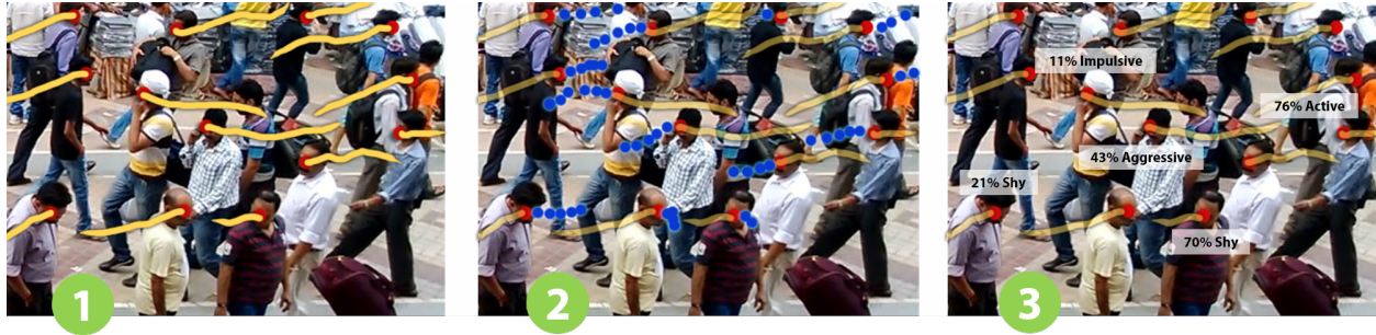
Figure 1.2: Overview: We highlight the different aspects of movements (tracked trajectories marked with yellow in (1), predicted trajectories as blue dots in (2) and personalities/behaviors in (3)) of pedestrians in the same scene.
