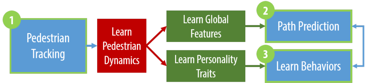
Figure 1.4: Overview: In this thesis, we present several interactive algorithms to extract pedestrian trajectories from videos in dense crowds. Our approach combines different pedestrian motion models with particle tracking and a mixture of motion models. We compute the pedestrian dynamics (a collection of different behavior and movement patterns, (Kim & Bera et al. 2014)) from these trajectories using Bayesian learning techniques and combine with global methods for long-term pedestrian prediction in dense crowds. Finally, we combine these techniques with Personality Trait Theory from Psychology to automatically classify the dynamic behavior or personality of a pedestrian based on his or her movements in a crowded scene. The resulting methods are robust and can handle sparse and noisy trajectories. We demonstrate the benefits of our long-term prediction and behavior classification methods in dense crowds and highlight the benefits over prior techniques.
