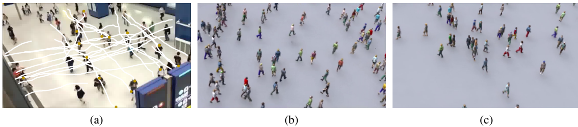
Figure 5.8: Augmented Crowd Rendered in a 3D Environment (a) Original Dawei video dataset with tracked trajectories, from which 27 trajectories are extracted; (b) Rendered scene with real and randomly inserted virtual pedestrians with similar trajectory-level behaviors, in which 100 virtual pedestrians have been added; and (c) Rendered scene with real and virtual agents using our behavior-learning approach.
