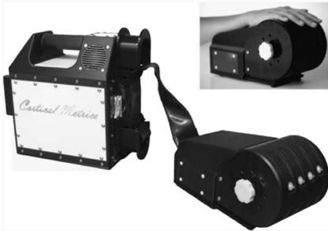
Figure 2.1 Four site vibrotactile stimulator. Top right: During an experimental session, subjects sit comfortably in a chair with their arm resting on an arm rest that is attached to the head unit of each device.
