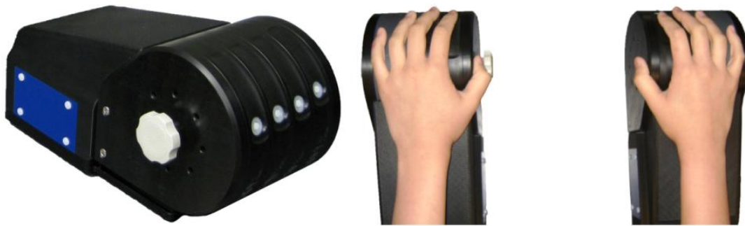
Figure 5.8 Bilateral modifications to stimulator placement. So that the bilateral conditions could stimulate both hands simultaneously, the device cabling was modified so to use two stimulators. Left: CM-4 Stimulator. Right: Overhead view of left and right hands positioned on two head units for the bilateral protocols.
