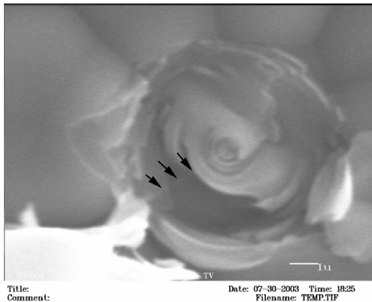
Fig. 3.2.2 SEM image of the cross section of a fractured carbon fiber. A single carbon nanotube (indicated by dark arrows) extrudes from the center of the carbon fiber.
