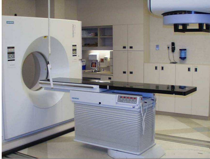
Figure 3.3: In-treatment-room CT scanner. A CT-on-rails (left) shares a treatment table with the linear accelerator (top right) that is used for external beam radiation therapy. This setup allows the patient to be imaged and treated in the same position.
