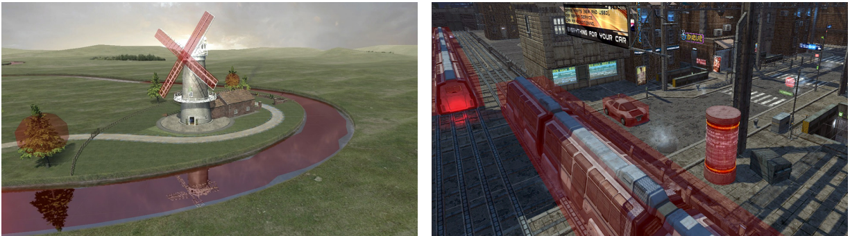
Figure 5.3: This visualization shows the sound sources for the windmill and city scenes in red. In the windmill scene, box sound shapes are used to represent the windmill sails, spheres are used for trees, and a triangle mesh is used for the nearby river. In the city, the train and car sound sources are represented by boxes, while scrolling advertisements are represented using meshes that correspond to the visual geometry.
