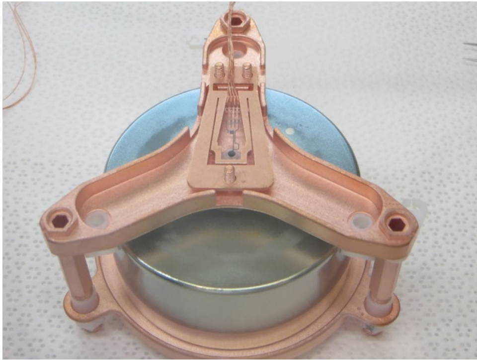
Figure 1.5: A photograph of a detector unit in the MAJORANA DEMONSTRATOR. Note, the detector unit is upside-down relative to Fig. 1.4.
