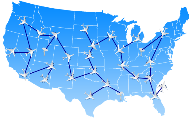
Figure 3.3: A pictorial representation of the connection of aircraft into a mesh network and to ground station gateways.
