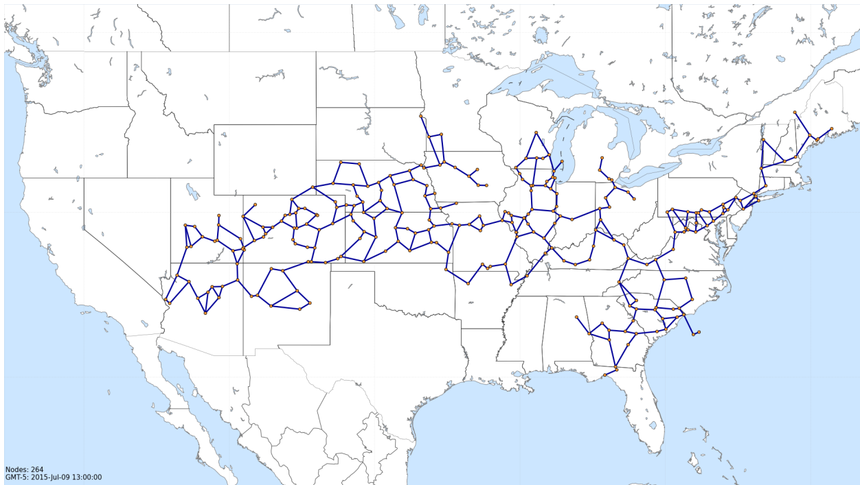
Figure 5.9: A snapshot of the initial network of aircraft used for the single high-rate flow experiments and the all pairs experiments. The 264 nodes shown here span a large portion of the United States at 1:00 p.m. on Thursday, July 9, 2015.
