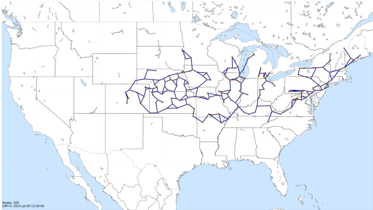
Figure 4.24: The network of aircraft used for the dynamic node simulation. A subset of 200 aircraft over the United States at 1:00 p.m. July 9, 2015.
