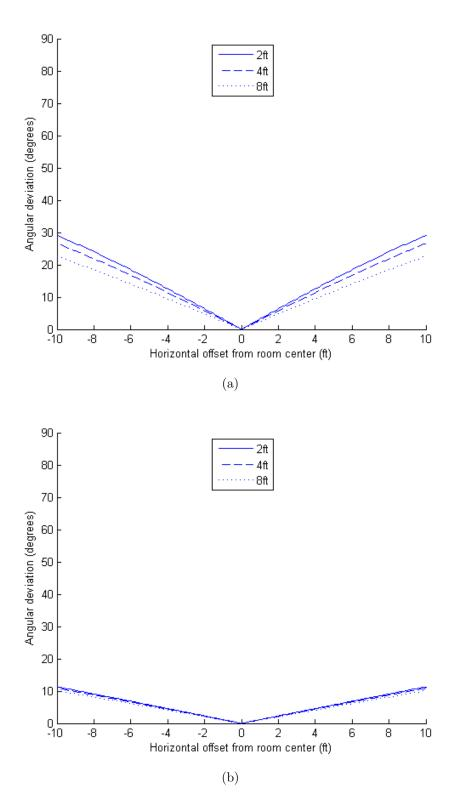
Figure 4.4: The gaze error for virtal cameras (a) 16' and (b) 48' behind the display wall, as shown in Figure 4.2(b). The axes and line sets are the same as in Figure 4.3.
