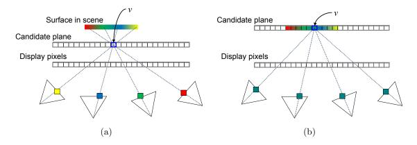
Figure 4.8: Plane sweeping comparisons: For a voxel v in the candidate plane in (a), the four cameras would see different colors, making it unlikely that there is a surface in v. In (b), all cameras see the same color at v, giving a higher likelihood of a surface.
