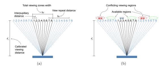
Figure 5.3: Repeating viewing zones in a regular barrier display: (a) shows the spacing of repeating zones; (b) shows the regions of conflict between viewers.
