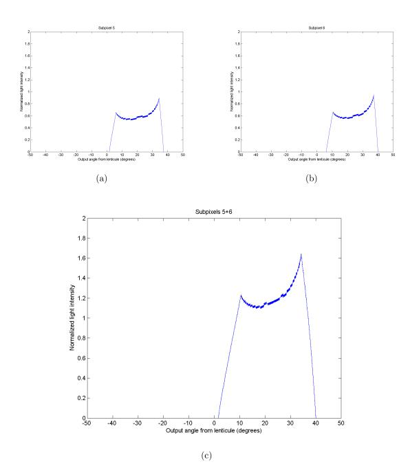
Figure 5.21: Energy from (a) subpixels 5 and (b) 6 by angle, normalized by the peak energy of all subpixels. (c) Combined light energy for subpixels 5 and 6.
