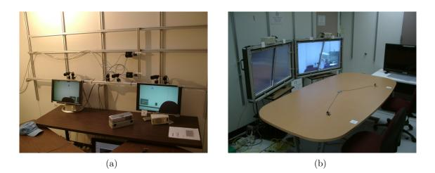
Figure 5.15: The half-duplex capture and monoscopic multi-view display system. (a) shows the capture configuration, with two camera per viewpoint, corresponding to viewer positions A and B at the display site and an additional central camera pair for comparison purposes. (b) shows the two monoscopic multi-view displays for viewers in positions A and B.
