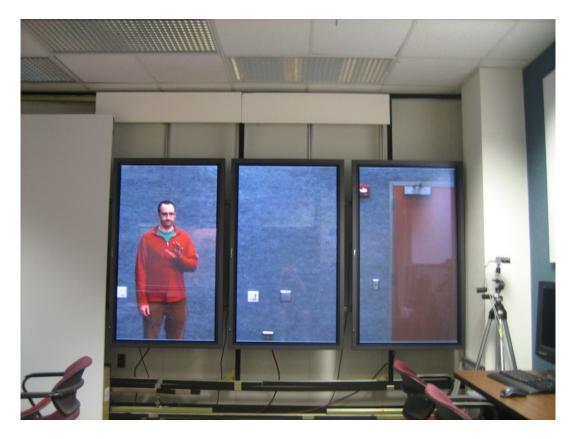
Figure 4.21: A photograph of video silhouette imagery shown on the telepresence wall displays.
