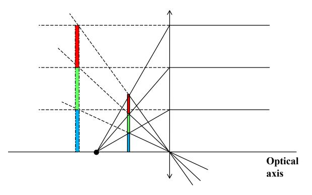
Figure 5.6: Expansion of the ray diagram for an RGB subpixel triplet.
