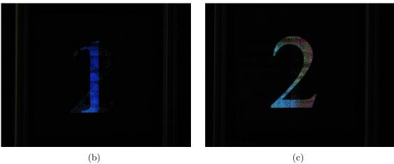
Figure 6.8: Two masked images are blended to form the (a) output image sent to the display. Photographs from the (b) left and (c right eye positions of a viewer centered 1 m from the display.
