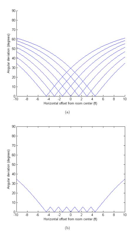
Figure 4.26: The gaze error for 7 cameras located at 1.5' intervals at the display, with a user at 8'. The gaze error for each camera is shown separately in (a), and the combined minimum gaze error for the system is shown in (b).
