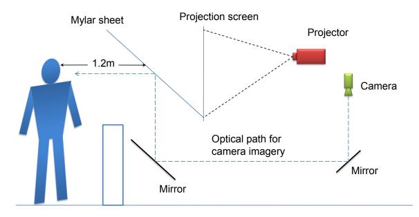
Figure 2.3: A profile view of the geometry of France Telecom's 'magic wall' telepresence system, showing the semi-reflective mylar sheet, through which the viewer sees the projected imagery of the remote site, and which reflects the telephoto camera image.
