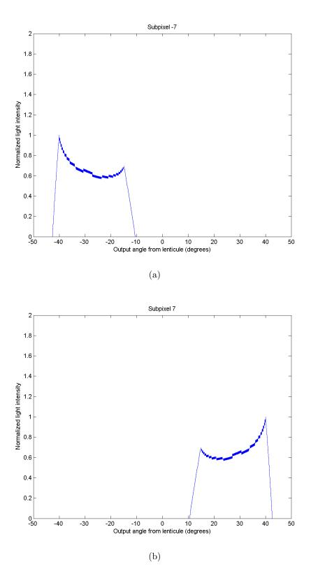
Figure 5.20: Energy from (a) subpixels -7 and (b) 7 by angle, normalized by the peak energy of all subpixels.
