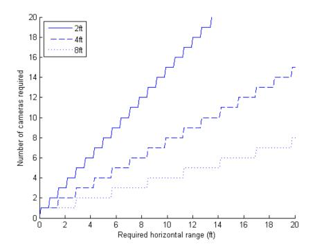
Figure 4.28: The number of cameras required to ensure a  $10^{\circ}$  maximum gaze error for a given horizontal distance, calculated by Equation 4.7. The three lines correspond to 3 different z offsets, with the user at 2, 4, or 8 feet from the display.
