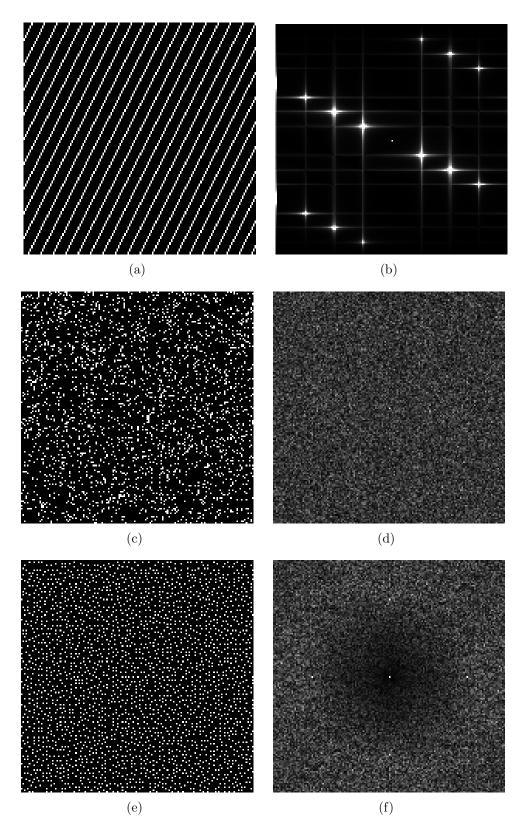
Figure 6.2: Fourier transforms of barrier patterns: (a) Regular barrier pattern; (b) FFT of (a). (c) Random pattern; (d) FFT of (c). (e) Poisson disk distribution pattern; (f) FFT of (e).
