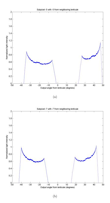
Figure 5.23: Light energy from (a) subpixel -5 and the corresponding -5 subpixel in the neighboring lenticule, and (b) subpixel -7 and the corresponding -7 subpixel, normalized by the peak energy of subpixels under the primary lenticule.
