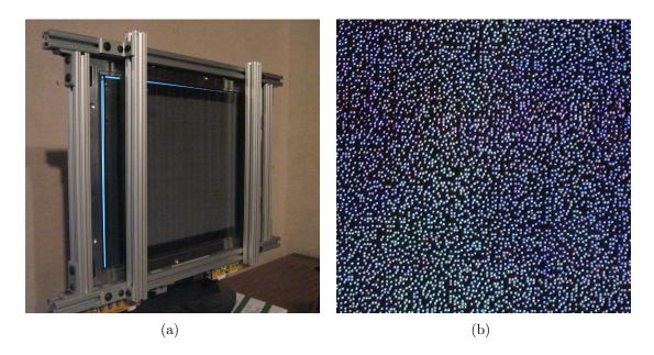
Figure 6.6: Views of the RHD prototype: (a) the barrier fixed in front of the LCD panel, and (b) a photograph of a small part of the actual barrier in front of the fully lit display panel.
