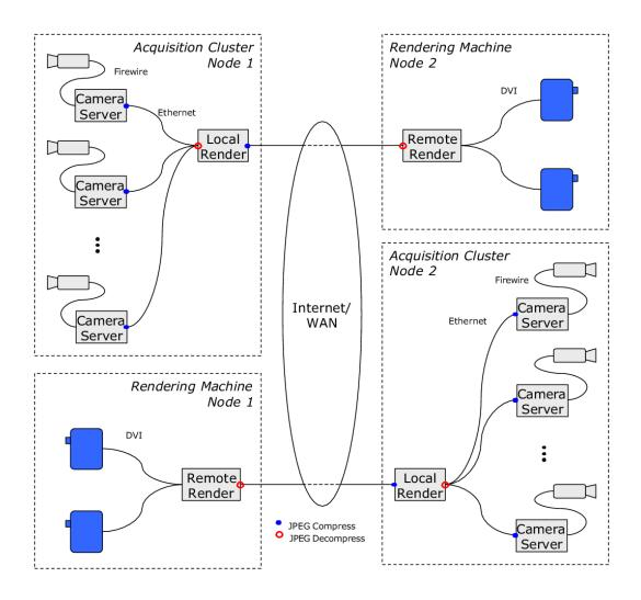
Figure 3.7: The system architecture of our prototype.
