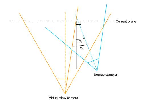
Figure 4.9: Weighting angles between the source camera, virtual view camera, and normal to the current candidate plane:  $\theta_P$  is the angle between the source camera and plane normal, used for surface probability determination.  $\theta_C$  is the angle between the source camera and virtual view camera, used for color weighting.
