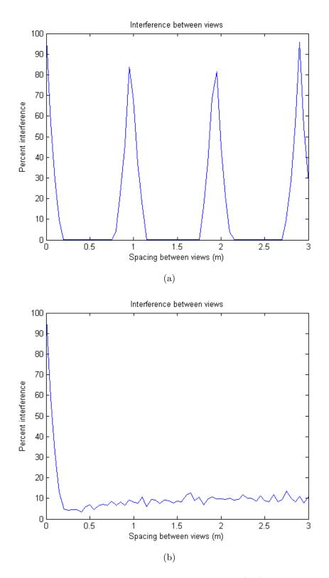
Figure 6.3: Interference between two viewers, one fixed at (1,1) as the second viewpoint moves horizontally from 0 to 3 m away at the same distance: (a) regular barrier of a conventional autostereoscopic display, and (b) randomized barrier.
