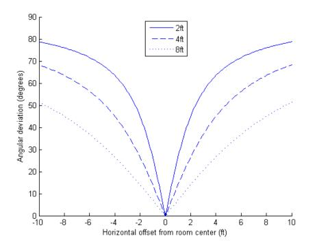
Figure 4.3: The gaze error for a panoramic camera at the display wall, as shown in Figure 4.2(a). The horizontal axis indicates the horizontal (x) offset between the user and camera, and the vertical axis shows the gaze error in degrees. The three lines correspond to 3 different z offsets, with the user at 2, 4, or 8 feet from the display.
