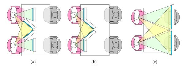
Figure 5.1: Potential multi-viewer display configurations. (a),(b) present unique views to each user with separate monitors. (c) represents the use of multi-view displays.
