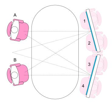
Figure 5.13: The prototype two-on-four teleconferencing scenario. Participants A and B are local. The four remote participants are shown on two large multi-view displays that provide unique views to A and B.
