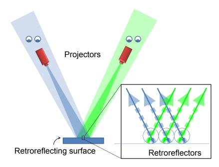
Figure 2.7: Retroreflective surfaces reflect light rays along their incident path. The light from a projector will return in the direction of the projector.
