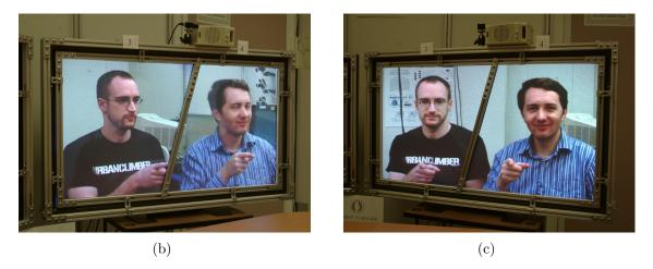
Figure 5.16: The remote participants at 3 and 4 are pointing at the user in position B. The multi-view display presents simultaneous views to different locations: (b) shows the view of the remote users from position A, and (c) shows the view from position B.
