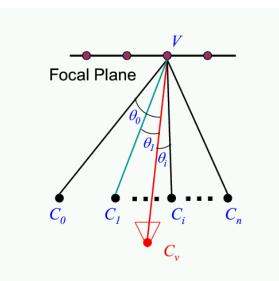
Figure 3.4: Angles between desired view camera  $C_v$  and texture cameras  $C_{0..\kappa}$ , at a vertex V on the focal plane.
