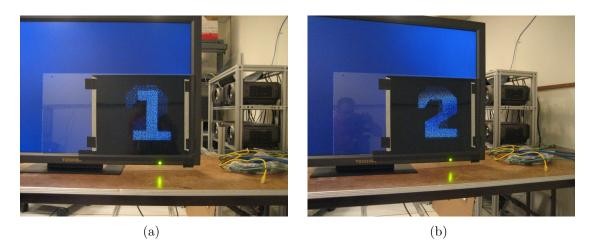
Figure 6.5: Film barrier test shows significant ghosting between views.
