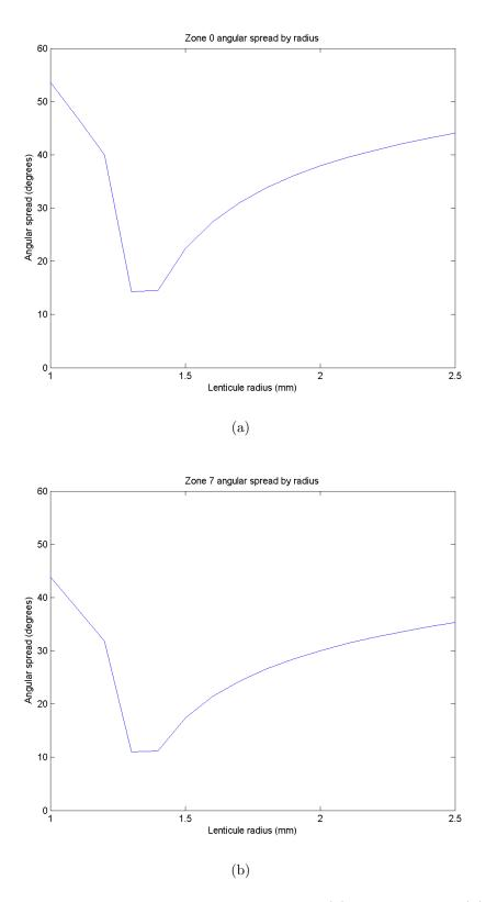
Figure 5.25: Angular viewing zone spread by radius for (a) subpixel 0 and (b) subpixel 7. The minimum values corresponds to a focal length close to the distance to the subpixels.
