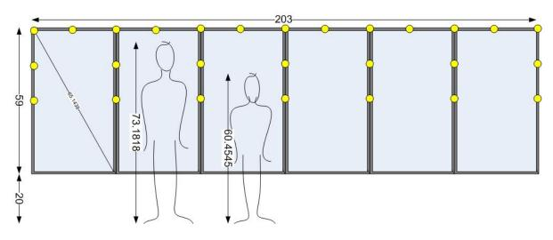
Figure 4.1: A prototype sketch of the display layout for a six panel telepresence wall. The yellow circle represent camera positions around the displays. Used with permission from J. William Mauchly, Cisco Systems.
