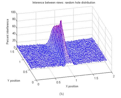
Figure 6.4: Interference between viewers, one fixed at (1,1) and the other at the plotted (x,y) position: (a) regular barrier of a conventional autostereoscopic display, and (b) randomized barrier.
