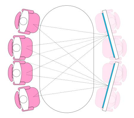
Figure 5.11: The four-on-four teleconferencing scenario goal includes four remote users depicted on two large multi-view displays that provide unique views to each of four local viewers.
