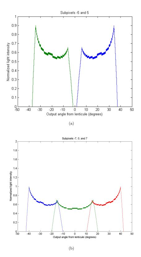
Figure 5.22: Light energy from (a) subpixels -5 and 5 and (b) -7, 0, and 7 by angle, normalized by the peak energy of all subpixels.
