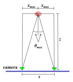
Figure 4.27: Given a maximum allowed gaze angle  $\theta_{max}$ , the optimal camera spacing s is equivalent to twice the maximum horizontal offset  $x_{max}$ .
