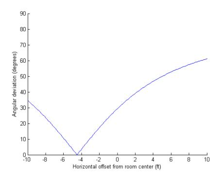
Figure 4.25: The gaze error for a single camera at the display wall, offset from center by 4.5', for a user at 8'. The horizontal axis indicates the horizontal (x) offset between the user and camera, and the vertical axis shows the gaze error in degrees.
