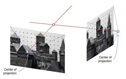
Figure 2.4: Depth from stereo correspondences in a pair of images. Rays from two cameras through similar image regions can be triangulated to find object depths.
