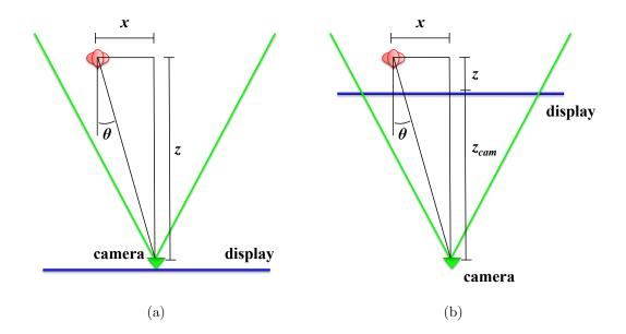
Figure 4.2: Top-down view of geometry for calculating gaze error of a remote participant at offset (x, z). The gaze error  $\theta$  is the angular difference between their actual viewing direction and the apparent viewing direction due to the capture camera offset. (a) shows the gaze error for a camera located at the display, and (b) shows the gaze error for a camera located at  $z_{cam}$  behind the display.
