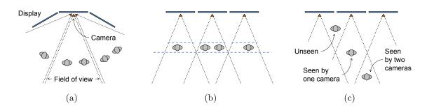
Figure 4.17: Top-down diagram of camera fields of view: (a) A shared center of projection and aligned fields of view prevent overlap between camera images. (b) Front facing camera systems sometimes restrict the usable area to prevent multiple images. (c) There are regions where people or objects will not been seen by any camera, or are visible in one or more cameras.
