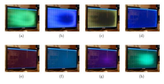
Figure 5.2: The Newsight 40" autostereoscopic display simultaneously provides 8 different views, spaced every 6cm, at 4m from the display.
