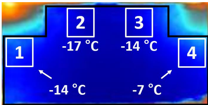
Figure 5.8. Thermal images of base Peltier at 5.1 A showing new mounting locations for the valves (outlined in white). The temperature of the base Peltier at each mounting location is noted. The region outlined in black is covered with pyrolytic graphite.
