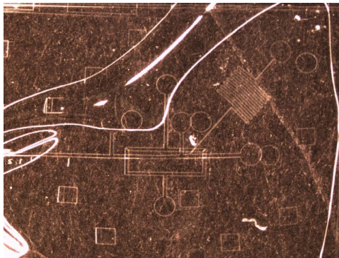
Figure 15. Two layers not bonded and shifted when removed
