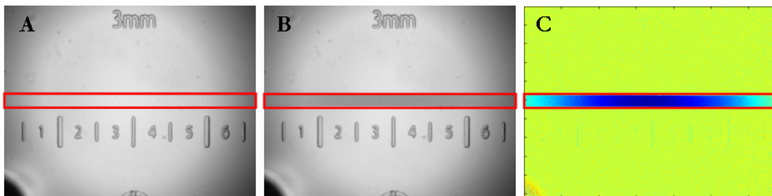
Figure 25. Extracting percent of light transmission. A. Baseline - channel empty B. Plug centered in view C. Percent of light transmission
