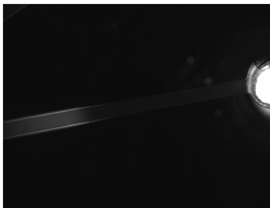
Figure 23. PDMS fluorescing where parylene coating is not present
