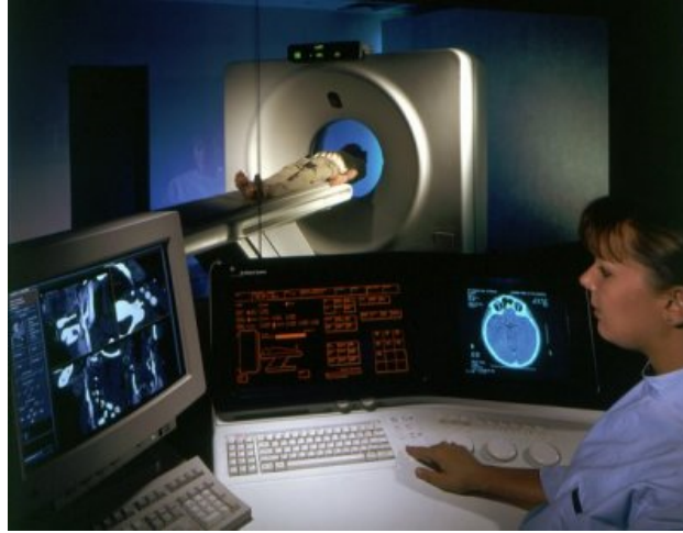
Figure 1.3: A CT scanner where a three dimensional image is reconstructed of an object from multiple projections images taken from different viewing angles. Image reproduced from ( http://www.daviddarling.info/encyclopedia/C/computed_tomography_scanning.html )
