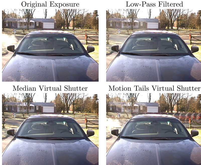
Figure 5.7: An input frame from the car defrosting sequence and three different output exposures from the virtual shutter with varying characteristics. The low-pass results washout regions where the car’s exhaust appeared, while the median virtual shutter result removes the exhaust. The motion tails output shows the combined exhaust of multiple frames plus evidence of an SUV driving by.
