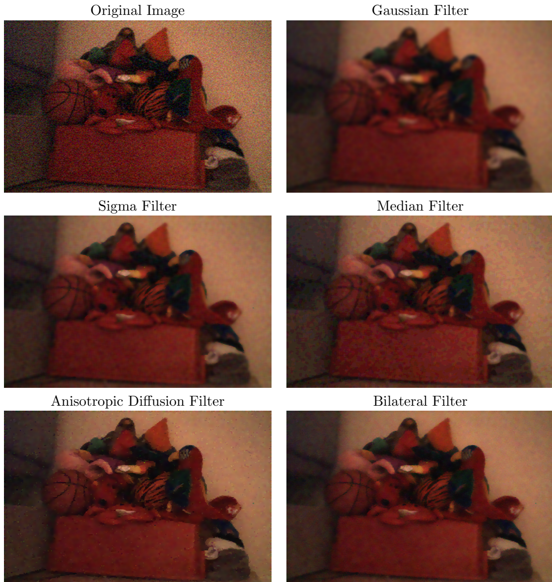
Figure 2.2: Comparison of existing spatial filtering techniques. The original image exhibits a high noise level in both luminance and chrominance. The Gaussian filter ( \sigma = 5.0 ) blurs the edges but removes the noise. The Sigma filter ( \sigma = 30 ) preserves some of the edges but corruption begins to occur at this \Omega kernel size (11x11). The 11x11 median filter preserves many edges, but introduces new distortion in blotchy regions. Anisotropic diffusion (50 iterations with K = 7 ) does an excellent job, save some stray pixels in the background. The bilateral filter ( \sigma_h = 5 and \sigma_i = 30 ) also does an excellent job filtering in a single pass with very smooth regions within objects.
