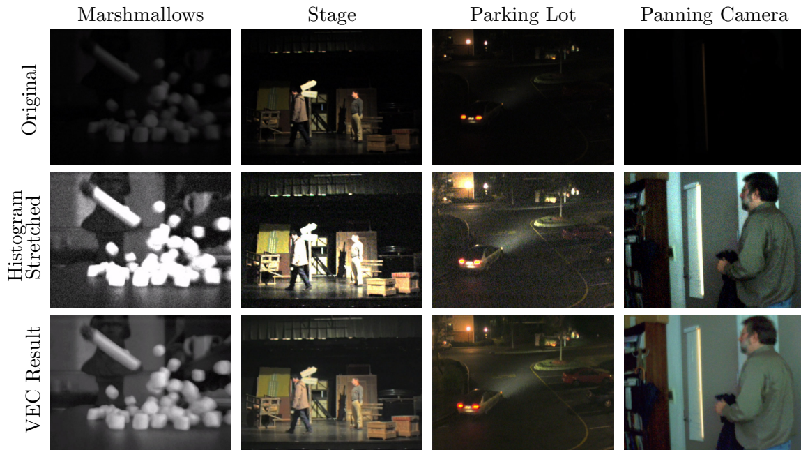
Figure 4.11: Images of four LDR videos with no enhancement, with histogram stretching, and after being run through the VEC system. The marshmallows video shows a dart hitting a stack of marshmallow, filmed at 120 fps. The second shows people walking around a stage. This video is an excellent example of a “peaky” histogram where a few image elements are well exposed, but nothing else is. The third shows a nighttime surveillance video of a parking lot. Finally, a video with a moving camera is shown, enhanced using video shearing to align samples spatially between frames.
