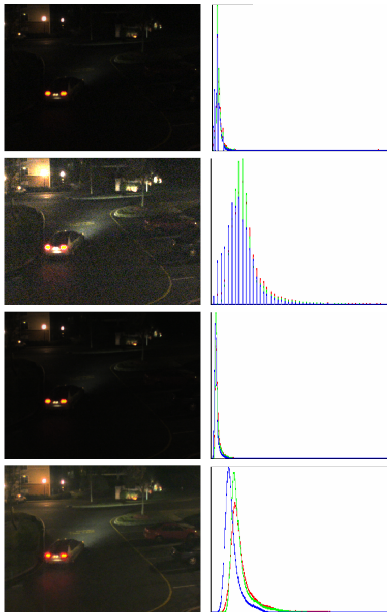
Figure 4.10: Inspection of color histograms in the VEC process. From top to bottom: the original video frame and its histogram; a histogram stretched frame and its histogram showing quantization error; an ASTA processed frame and its histogram which is similar to the unfiltered histogram; the tone mapped ASTA frame and its stretched histogram without quantization error. Note that the vertical scale in these histograms is separately stretched to show maximum detail in each.
