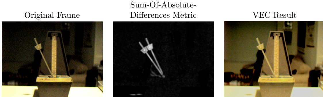
Figure 4.4: Illustration of the spatial neighborhood dissimilarity value used in temporal filtering. The original frame is shown on the left. Each (x,y) for a pair of nearby frames are shown in the middle image. Two metronome arms are seen because the dissimilarity value is based on absolute value. The right image is the same frame processed using VEC with both ASTA and the tone mapper.
