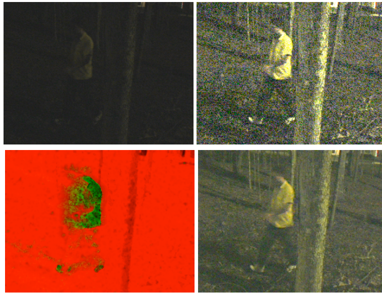
Figure 4.8: A frame from a video processed using the VEC system. Upper Left: original frame; Upper Right: histogram stretched version; Bottom Left: red = number of temporal pixels integrated, green = number of spatial pixels integrated; Bottom Right: the VEC result after filtering and tone mapping.
