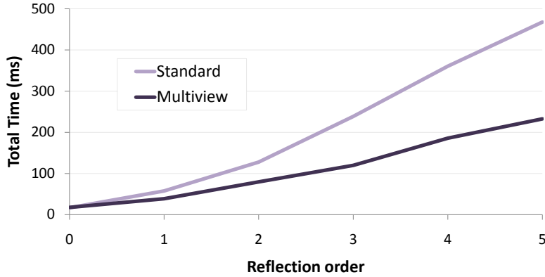
Figure 5.6: Multiview performance: Multi-view ray tracing outperforms standard ray tracing for scenes (80k triangle scene shown) with many specular views. The multi-view timings include the time cost of all necessary sorting and reordering.
