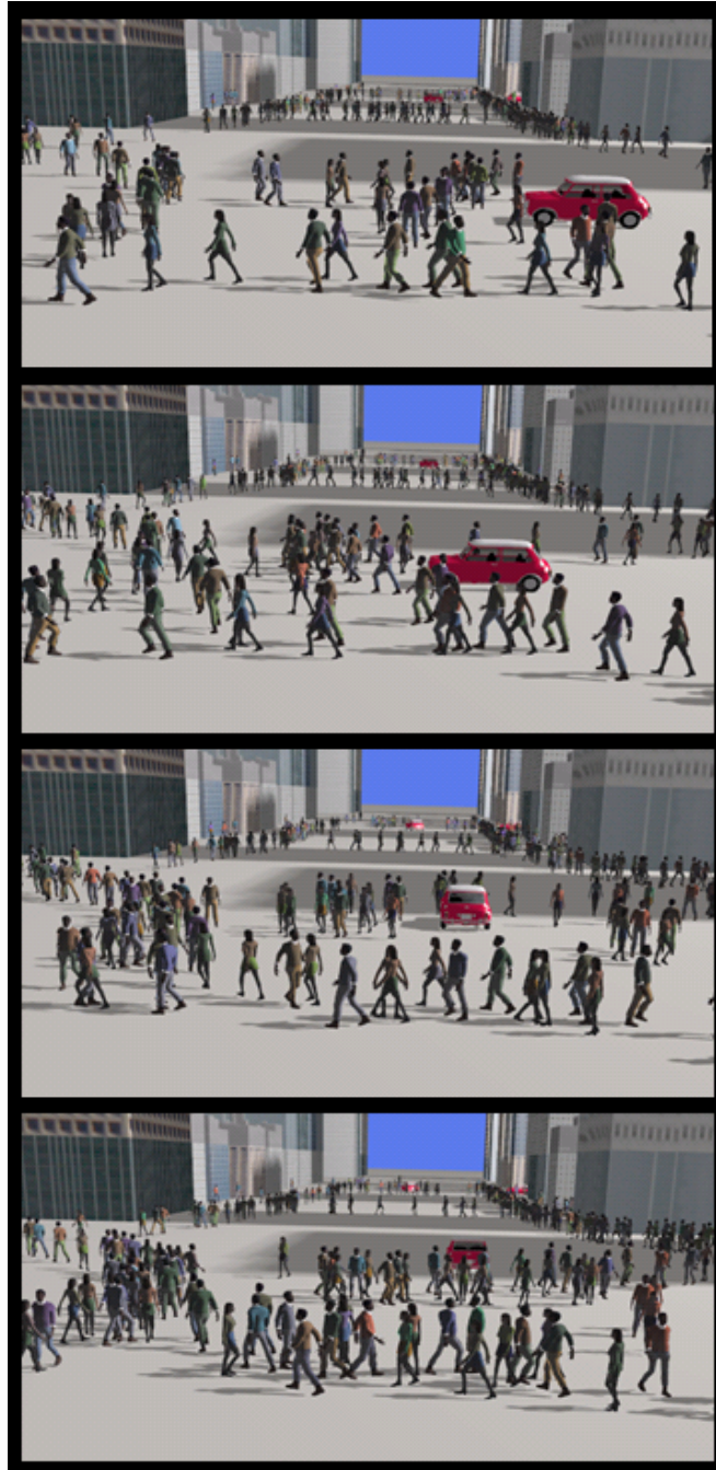
Figure 6.29: Crowd simulation in an urban landscape: A street intersection in a virtual city with 924 buildings, 50 moving cars as dynamic obstacles and 1,000 pedestrians. We show a sequence of four snapshots of a car driving through the intersection. As the car approaches a lane of pedestrians (top), the lane breaks (middle two images) and the pedestrians re-route using alternate links on the adaptive roadmap. Once the car leaves the intersection (bottom) the pedestrians reform the lane using the adaptive roadmap. We are able to perform navigation of 1,000 pedestrians in this extremely complex environment at 54fps on a 2.6Ghz Dual Processor PC.
