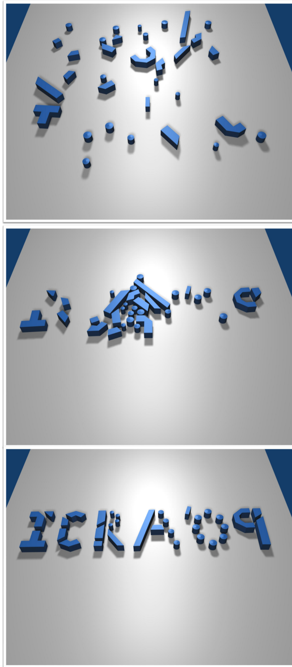
Figure 6.23: Letters: The letters benchmark consists of 33 convex and non-convex robots in an assembly-like situation. (a) The letters start off at random positions and orientations. (b) Repulsive and attractive forces allow the robots to move toward their goals but to also avoid collisions with each other. (c) The robots arrive at their final location.
