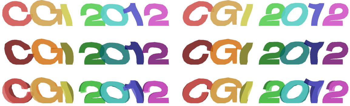
Figure 5.3: Example 2D shape deformations showing different results with different Poisson's ratios \nu (each column results from the same first-type boundary conditions); top: \nu = 0.1 ; middle: \nu = 0.49 ; bottom: comparison by overlaying the two results.
