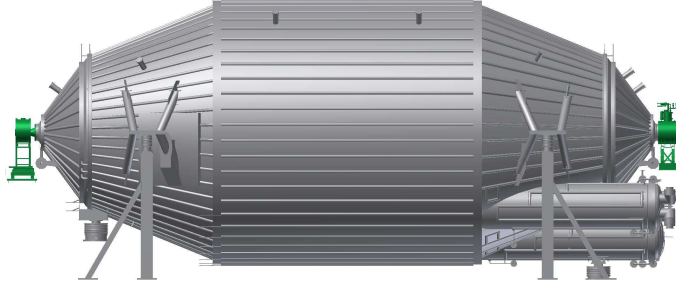
Figure 5.8: A diagram of KATRIN’s main spectrometer, with superconducting magnets (green) at its entrance and exit.
