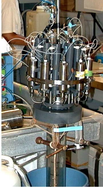
Fig. 5- 2: Picture of HYDRA on board ship. The stainless steel 7 mL sample chambers are shown in front of the 20 mL gray-PVC flush chambers. The probe tip is shown immersed in a water-filled plastic tube.
