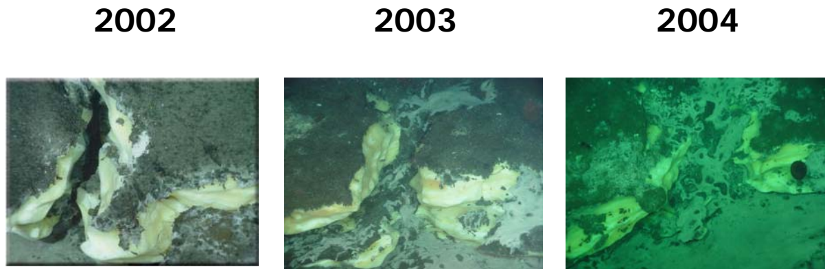
Fig. 4- 9: Annual photographs taken of outcropping hydrate at Barkley Canyon. In 2002, the valley between each hydrate slab was about 10 cm wide. In 2003, this valley widened to ~17 cm and in 2004, it grew to about 24 cm. Photographs courtesy of Ross Chapman, University of Victoria.
