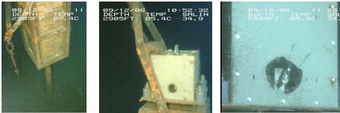
Fig. 3- 11: Seafloor photos of the PFA retrieval. A) The first sighting of the PFA showed it was standing upright and vertical about 2 meters out of the sediment. B) The OsmoSampler package shown with minimal biofouling and all parts intact. C) Although a little corroded, the high pressure valve was still intact.
