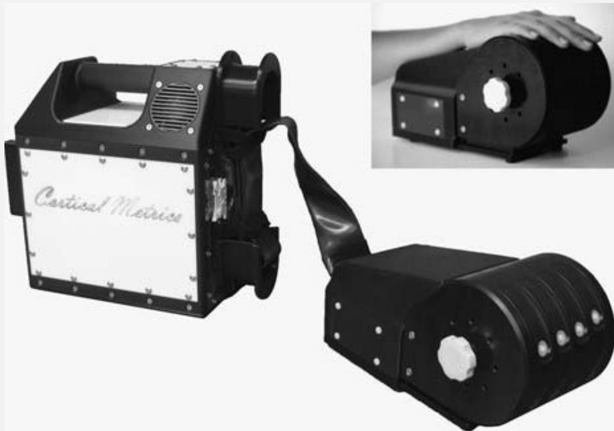
Figure 2.1: Four Site Vibrotactile Stimulator. Each of the four probe tips is positioned by rotating the four independently-positioned drums to maximize contact between finger pads and the stimulator tips. During an experimental session, subjects were seated comfortably in a chair with their arm resting on the arm rest attached to the head unit of the device. Digits D2 through D5 were then positioned for vibrotactile stimulation.
