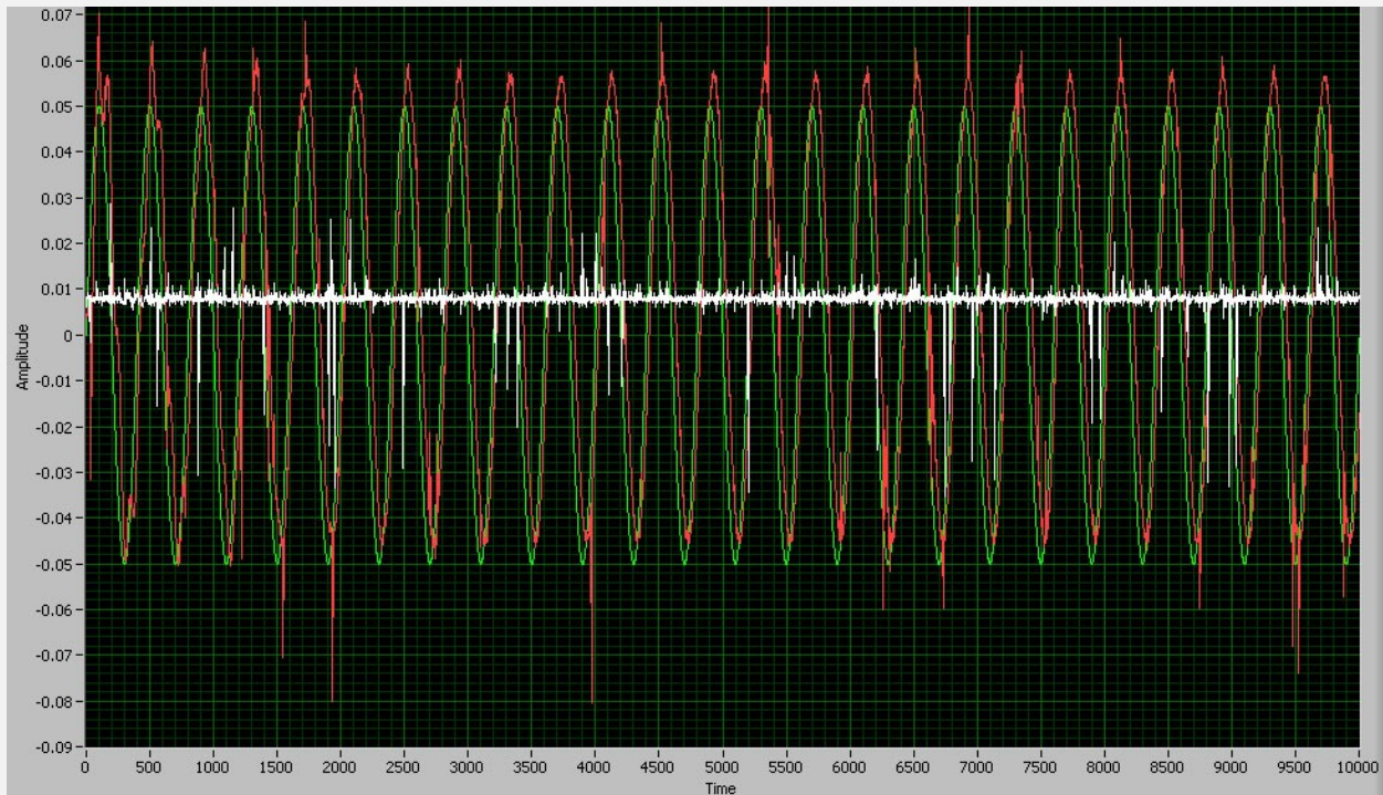
Figure 4.1: Optical Sensor Readings Verify Sinusoid Generation
