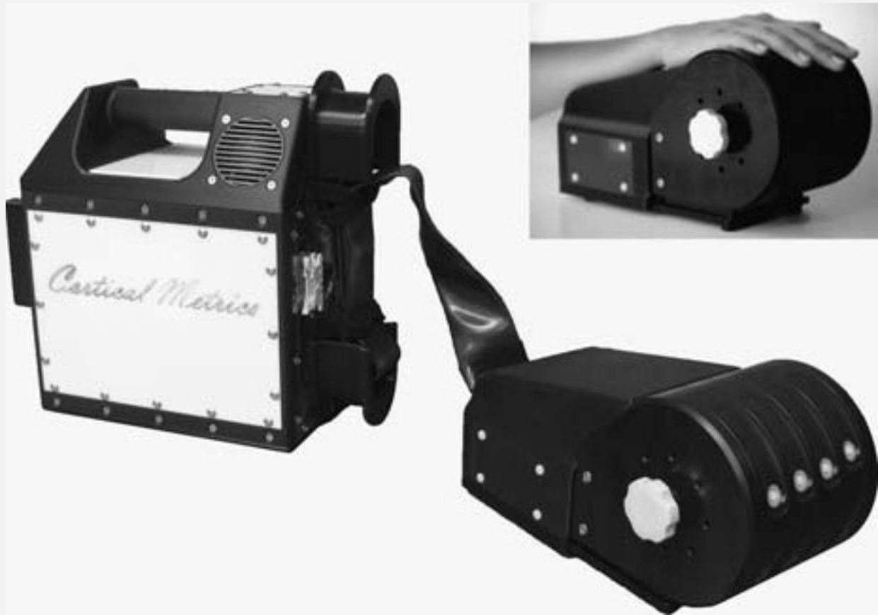
Figure 3.1: Four Site Vibrotactile Stimulator. Each of the four probe tips is positioned by rotating the four independently-positioned drums to maximize contact between finger pads and the stimulator tips. During an experimental session, subjects were seated comfortably in a chair with their arm resting on the arm rest attached to the head unit of the device. Digits D2 through D5 were then positioned for vibrotactile stimulation.
