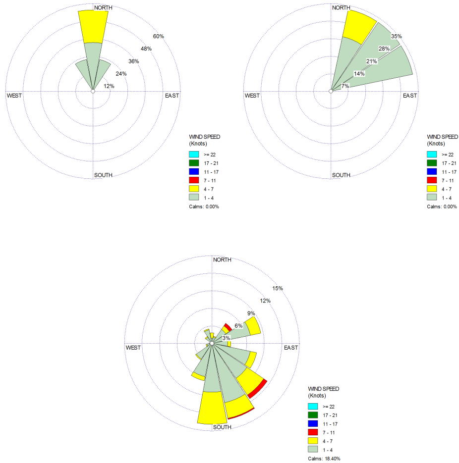
Figure A.7: Modeled surface wind direction and speed at the 12-km grid resolution for nighttime hours (0 to 8 GMT or 8 PM to 4AM LST) on June 6 (top left), June 7 (top right), and June and July (bottom).
