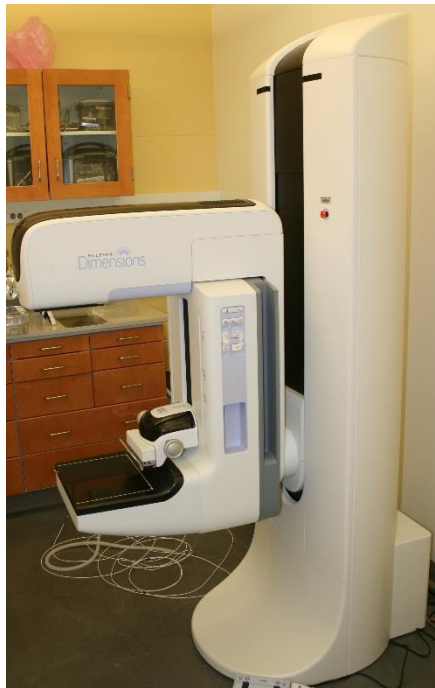
Figure 1.23 Photograph of a Hologic Selenia Dimensions DBT system in a laboratory setting.
