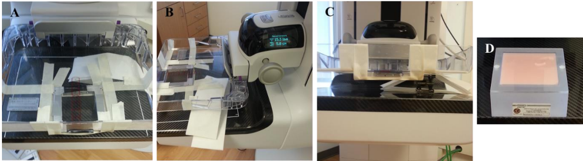
Figure 8.3 Photos of the experimental setup. (A) Top-view of the MTF cross-wire phantom attached to the breast compression paddle. A line pair phantom is also present. (B) Side-view of the setup showing the display on the gantry, used for relocating the paddle after each image. (C) Front-view showing the phantom suspended below the compression paddle. (D) ACR phantom, after the top and wax insert were removed, was used to level the compression paddle so that it was parallel to the detector surface.
