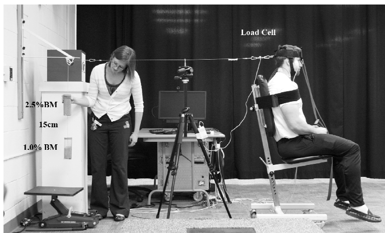
Figure 4.3. Example cervical perturbation set-up during forced extension.
