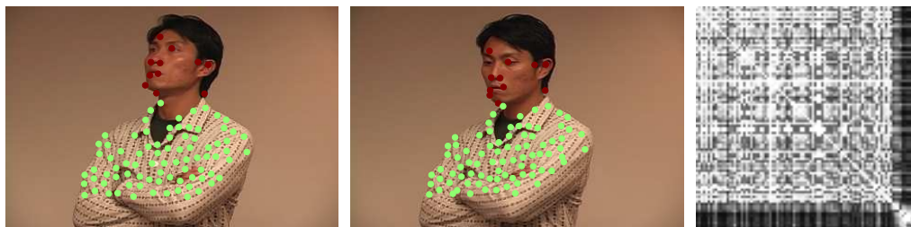
Figure 4.5: ( left and middle ) A sequence of a person moving with his head rotating around the neck. The color of a dot, red or green, shows the segmentation result. There is one misclassification, the red dot on the left shoulder. The other red dot on the left arm is an outlier. ( right ) The affinity matrix of locally estimated subspaces is shown. The row and columns are rearranged based on the segmentation.
