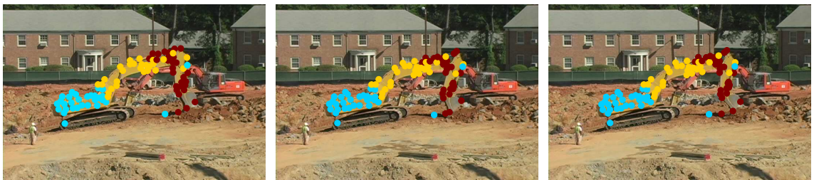
Figure 4.8: A sequence of a bulldozer with its upper-arm and forearm moving articulately around some axis. The color of a dot, red, blue or yellow, shows the segmentation result. There are 4 misclassification errors. Two are the yellow dots on the forearm and two are the red dots on the upper-arm. All of them are near the axis connecting both arms. Besides these, there are several outliers in the trajectories and they are clustered to one of the segments.
