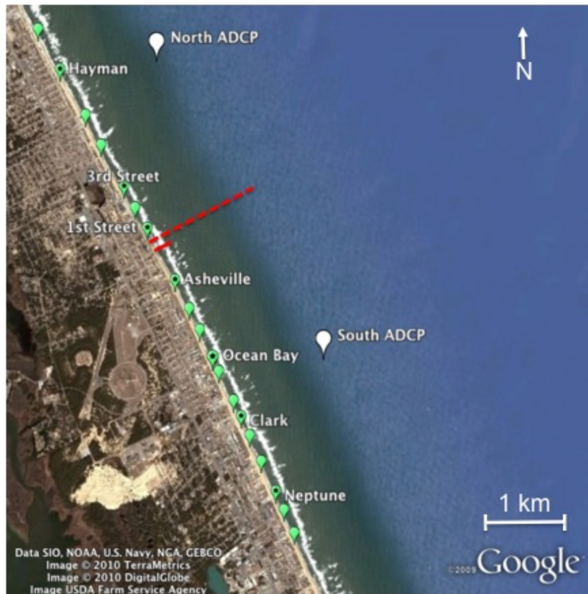
Figure 4.1 The study location at Kill Devil Hills, NC. The green marks show the location of the 19 lifeguard chairs, and black stars indicate the locations where surf zone bathymetry was monitored in 2008 and 2009. The red lines indicate the offshore extent of the RTK GPS (solid) and FRF (dashed) profiles. The white marks show the location of the 2 ADCPs deployed at roughly 12 m depth from June to December in 2008 and 2009.
