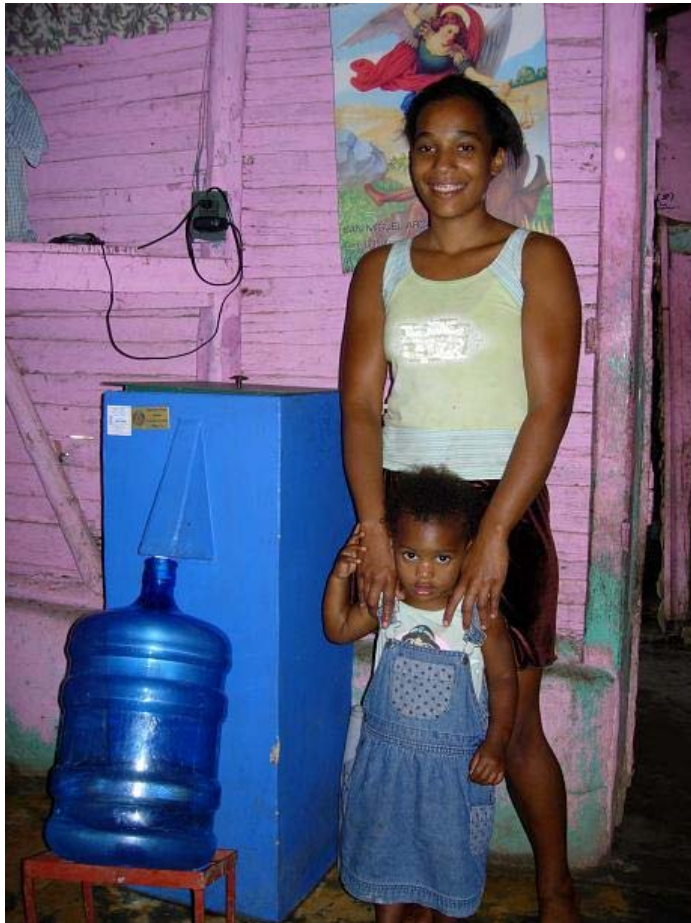
Figure 5.1 Biosand filter with base and water storage container in household in the KM 100 area of the Jayaco community
