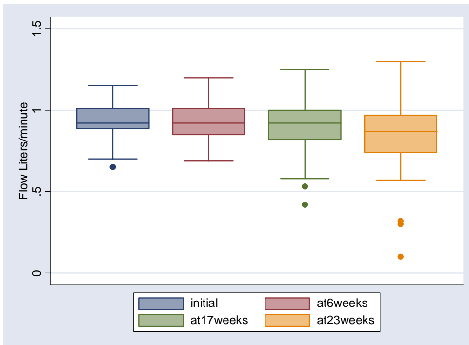
Figure 4.5 Flow rate of BSFs over time during six-month field trial in Bonao, Dominican Republic
