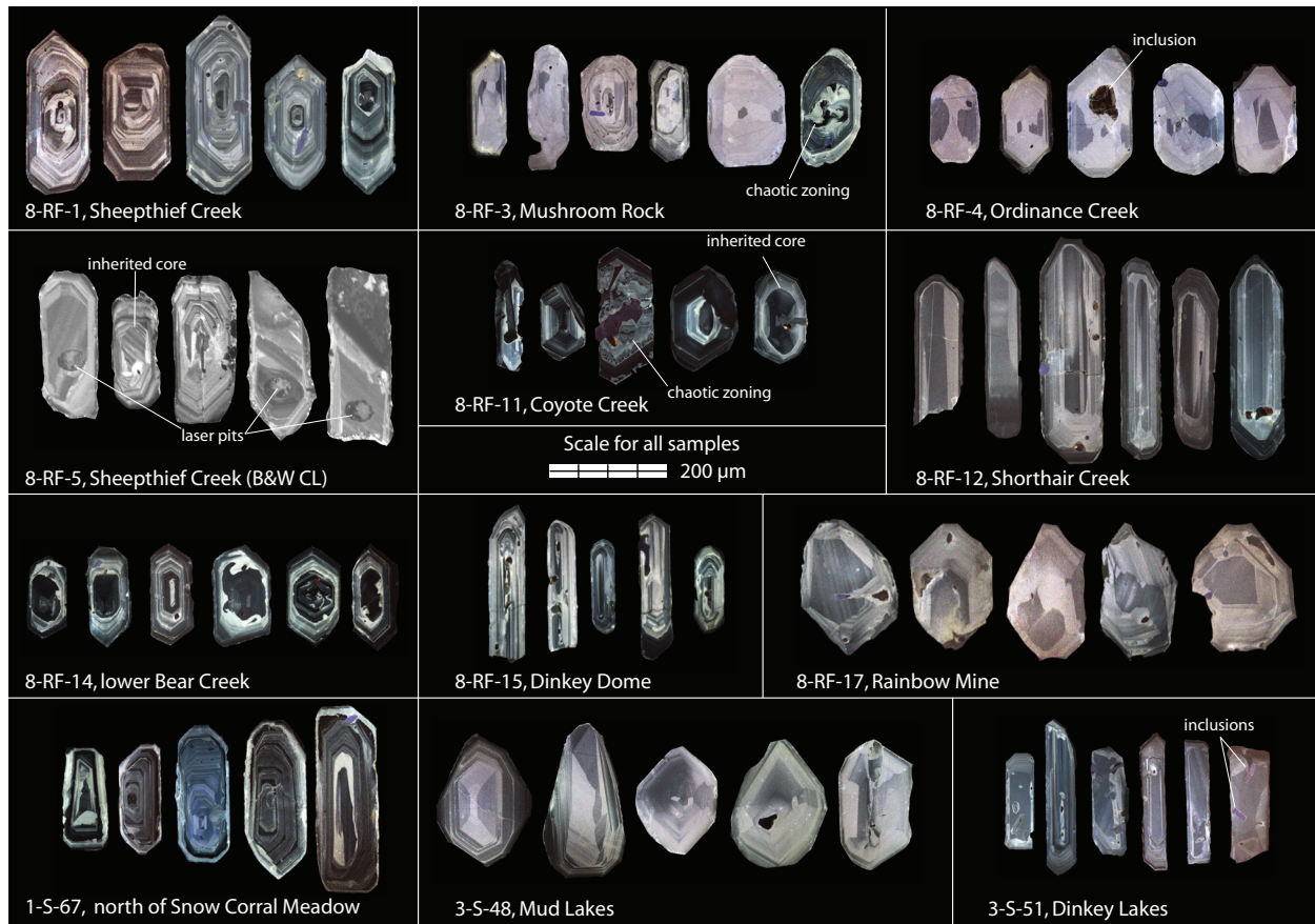
Figure 3. Cathodoluminescence (CL) images of representative zircons from dated samples. Most zircons have oscillatory or sector zoning, indicative of typical magmatic growth. Some notable features, such as inclusions or obvious inherited cores, are labeled. Images for all samples except 8-RF-5 are color CL collected at California State University – Bakersfield. Sample 8-RF-5 analyzed with black and white CL at Pomona College. Images for all samples are at the same scale.
