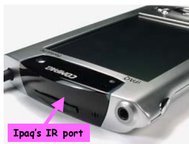
Figure 9. The IR port on the front end of the Ipaq for transferring data and controlling IR devices.
