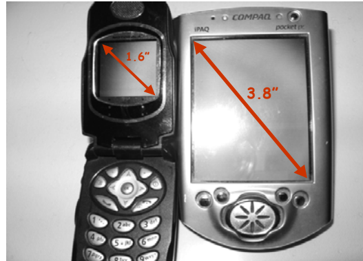
Figure 5. A depiction of cell phone (Motorola i710) and Pocket PC (Compaq Ipaq) screen size differences. The cell phone's screen is less than half of the Ipaq's.
