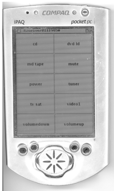
Figure 69. The receiver's history-based GUI on a single Ipaq screen. With the available space from filtering buttons, the remaining buttons can be stretched to fill the screen.
