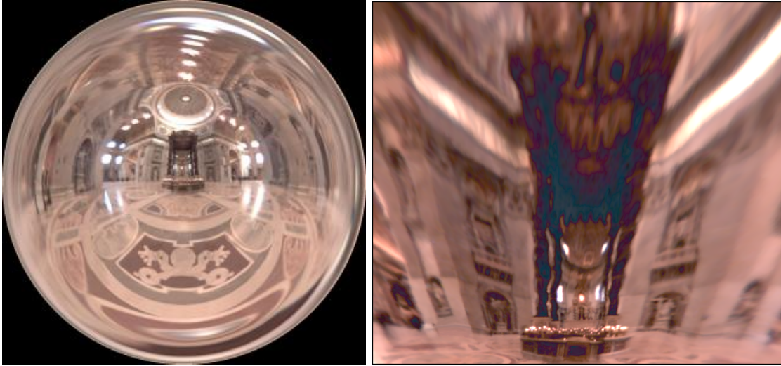
Figure 5.5: Mapping the virtual illumination environment to our physical setup. Left: The virtual lighting environment. Right: The image that is projected onto the screen. Note that the image is stretched upward and outward to represent the rays of light from the virtual illumination environment.
