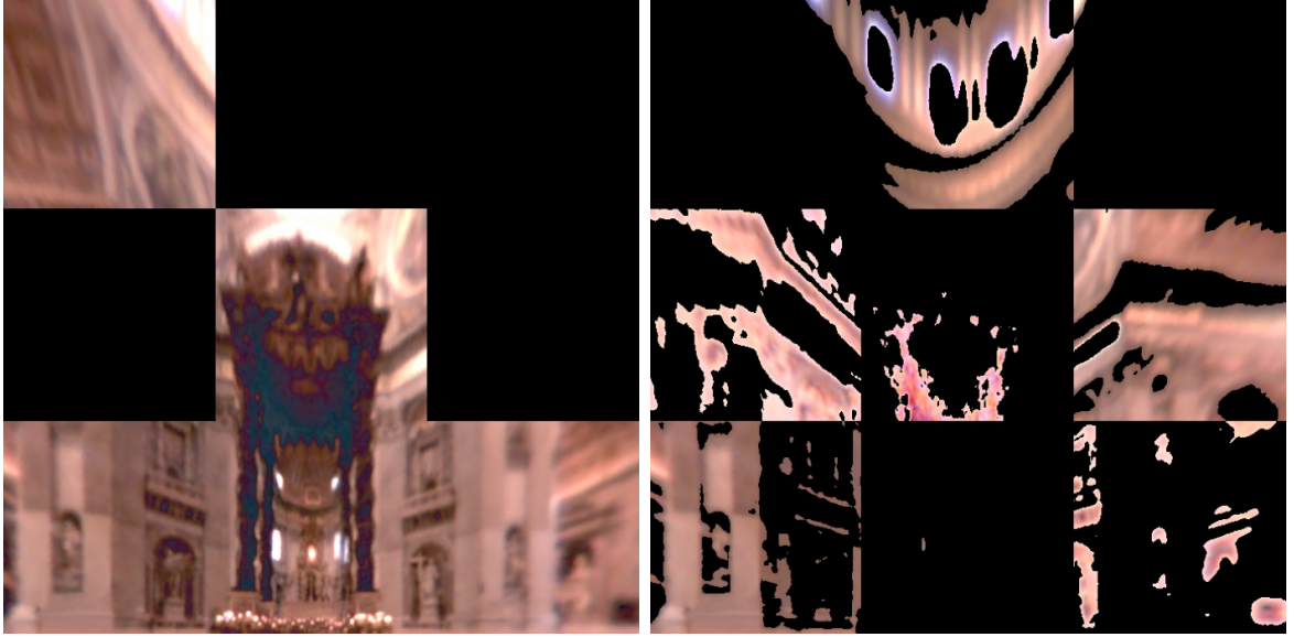
Figure 5.10: Multiplexing the St. Peter’s Cathedral light probe (light probe courtesy of debevec.org). Left: Low-dynamic range multiplexing. The screen is divided into 9 regions, where each region is either “on” or “off”. Approximately half of the regions are “on” at a time. Right: High-dynamic range multiplexing. Each region represents a different exposure level.
