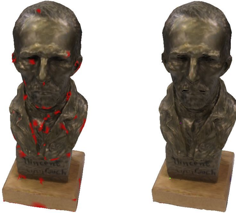
Figure 3.6: Left: The bust dataset with areas of missing data highlighted in red. Right: Imputation of the missing data fills in the areas with plausible values.
