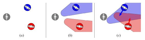
Figure 2.3: The union of multiple velocity obstacles can be an arbitrarily complex shape. (a) shows three agents. The grey agent plans with respect to the red and blue agents. (b) shows the truncated relative velocity obstacles. (c) shows the VOs displaced by the predicted velocities of their respective agents.
