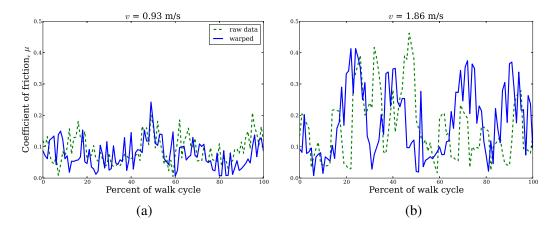
Figure 7.6: Minimum coefficient of friction. The two graphs show the minimum coefficient required to achieve the indicated gaits. (a) Trials 7\_04 and 7\_02 at 0.93 m/s. (b) Trials 7\_12 and 7\_02 at 1.86 m/s. The dashed green lines are from raw motion capture and the solid blue from synthesized motion.
