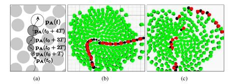
Figure 3.4: Authority: (a) An agent A and the trail (a sequence of trail proxies.) The trail proxies are placed at positions  $\mathbf{p}_i$ , at time instants  $t_0$ ,  $t_0 + T$ ,  $t_0 + 2T$ ,  $t_0 + 3T$  and  $t_0 + 4T$ . (b) A line of police maintains a formation while walking in a crowd; the police are associated with trail proxies and aggression proxies. (c) A simulation with the same initial configuration except without trail proxies.
