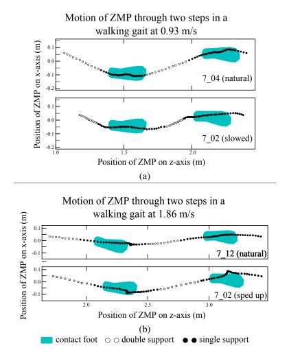
Figure 7.7: Trajectory of the ZMP. (a) 7\_04 at its natural speed of 0.93 m/s versus 7\_02 slowed to the same speed. (b) 7\_12 at its natural speed of 1.8 m/s versus 7\_02 at sped up to the same speed. The cyan markers represent approximations of foot position during ground contact.
