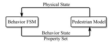
Figure 8.1: We simulate crowd behaviors appropriate to the Tawaf by coupling a high-level finitestate machine (FSM) with a low-level pedestrian model. The FSM computes behavior-state and property-set values for each agent. The pedestrian model, in turn, updates the agent's physical state.
