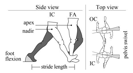
Figure 7.2: Five dominant, spatial gait properties. Each varies with stride length. How these properties change with respect to stride length are parameterized and serve as the basis for transforming one walking clip into another at a different speed.
