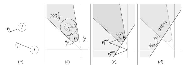
Figure 2.4: ORCA (a) Two agents, i and j, with velocities  $\mathbf{v}_i$  and  $\mathbf{v}_j$ , respectively. (b) The truncated velocity obstacle formed by agent j on i. (c) The computation of  $\mathbf{u}$ , the minimum change to relative velocity and the corresponding relative half-plane velocity obstacle. (d) The ORCA constraints.
