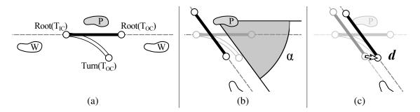
Figure 7.4: Illustration of how straight-line motion is mapped to turning. The swing foot is marked W and the support with a P. (a) the initial relationship between straight (black line) and curved (white line) trajectories. (b) the straight-line space is rotated around the support foot  $\alpha$  radians to point in the same direction as the velocity. (c) the space is translated by  $\vec{d}$  to so that the straight-line end point aligns with the ideal position.
