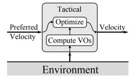
Figure 1.10: The architecture of a velocity obstacle tactical module. The environment, including nearby agents and obstacles, is used to define velocity obstacles. The preferred velocity and the velocity obstacles are used in an optimization algorithm to compute the final, feasible velocity.
