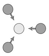
Figure 4.1: Force equilibrium. The sum of the repulsive forces on the active agent cancel each other out. The agent does not accelerate, although there are many directions it could travel to avoid collisions.
