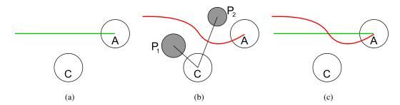
Figure 3.1: Responses of an agent A encountering a composite agent C. (a) The green line shows the original planned path taken by A. (b) In the presence of the proxy agent of C, A takes the red path and avoids collision with  $P_1$  and  $P_2$ . (c) Comparison of the paths.
