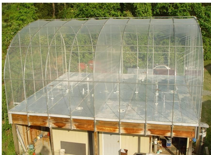
Figure 1. UNC Aerosol Smog Chamber
