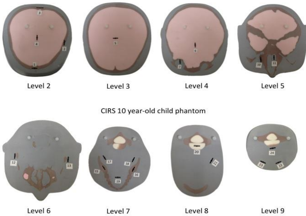
Figure 12B. Child ATOM Slices with machined OSL dosimeter locations
