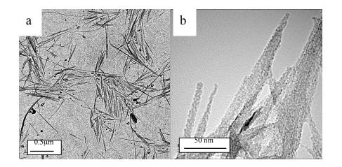
Figure 3.4: a) Low resolution TEM image of acid treated SWNT bundles before annealing to show the average bundle length is about 1 $\mu$ m, the scale bar is 0.5 $\mu$ m; b) High resolution TEM image of acid treated SWNT bundles, showing blurred edge of the bundles, indicating that they are wrapped with amorphous carbon after the acid treatment. The tapered ends also suggest that etching process happens both lateral and longitudinal.
