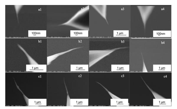
Figure 5.6 SEM images of CNT fibrils grown on commercial AFM probes while different  $\Delta t$  is applied. (a)  $\Delta t$  equals to zero, the probe is retracted right after it reaches the suspension;
