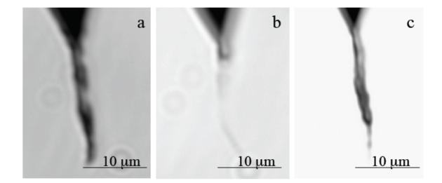
Figure 5.8 Optical images of CNT fibrils fabricated when different retraction speeds were applied. (a) Vr of 1 $\mu$ m/sec was applied; (b) Vr of 2 $\mu$ m/sec was applied; (c) Vr of 1 $\mu$ m/sec was first used then was changed to 2 $\mu$ m/sec, a continuous growth of CNT fibrils with different thickness was observed. The same CNT suspension, initial waiting time and AC voltage was used.
