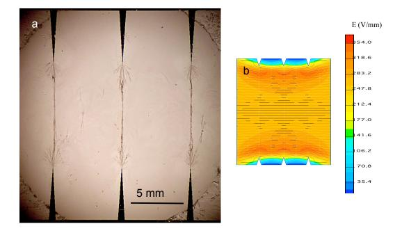
Figure 4.6 (a) Optical image of CNT fibrils assembled on facing electrode arrays. (b) Electrical field distribution of electrode array used in (a).
