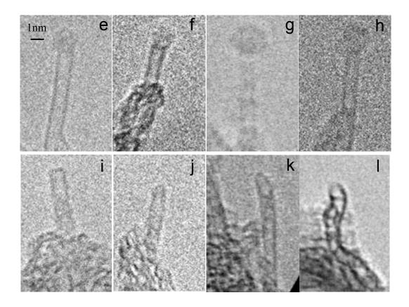
Figure 3.7 HR-TEM images of individual SWNTs after oxidation and annealing first at 400°C for 10hrs then at 800 °C for 1hr. (The figures share the same scale bar.)
