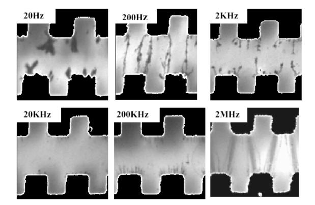
Figure 4.8 A series of optical images showing different CNTs structures formed under AC field with different frequency.
