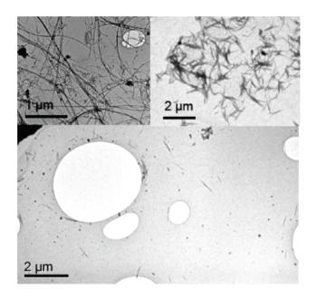
Figure 5.3 TEM images of CNTs used in this study. (a) Purified long carbon nanotubes; (b) Short nanotube suspension before centrifuge; (c) Short nanotube suspension after centrifuge.
