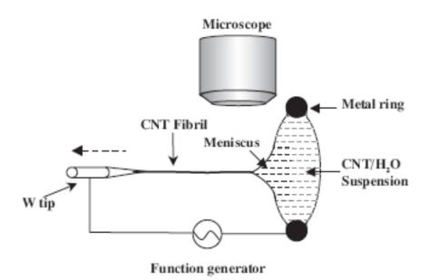
Figure 4.12 Schematic illustration of the dielectrophoresis process for assembly of CNT fibrils [21]
