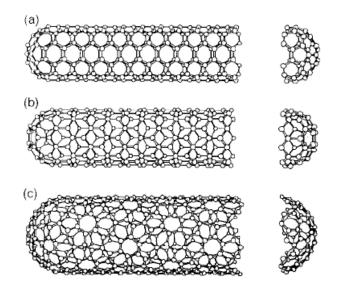
Figure 1.3 Different types of SWNT, (a) an armchair SWNT; (b) a zigzag SWNT; (c) a chiral SWNT [7]
