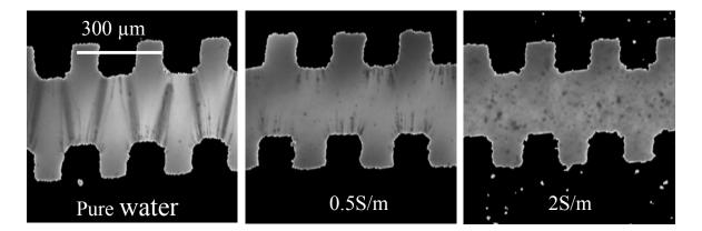
Figure 4.9 A series of optical images showing different structures CNTs formed under the same AC field but different ionic conductivity of the medium.
