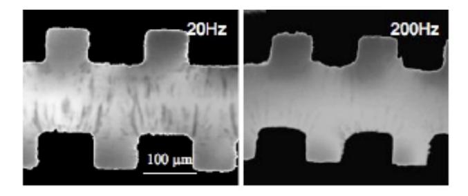
Figure 4.10 Optical images showing CNT structures form in viscous medium under different frequencies.
