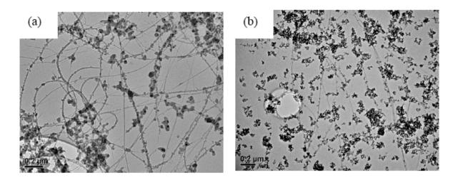
Figure 2.4 TEM images of as synthesized SWNT bundles. (a) SWNTs synthesized by laser ablation method using 0.3% Ni-Co target. (b) SWNTs synthesized by laser-CVD method using iron targe (99.99% purity from Alfar Asear), and 10% methane was added to the flowing gas while flow rate was 400 sccm.
