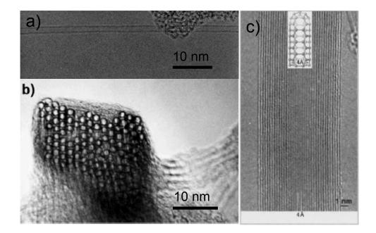
Figure 1.1 High resolution transmission electron microscope pictures of (a) An isolated SWNT [4] (b) Cross section of SWNT bundles. SWNTs produced by laser ablation and arc discharge bundles up because of van der Waals attration. The cross section forms a triangular lattice structure. The diameter of a bundle is between 10 and 50 nm, corresponding to 30-500 tubes per bundle [3]. (a) MWNT, the inner core can be as small as 0.4 nm [2].
