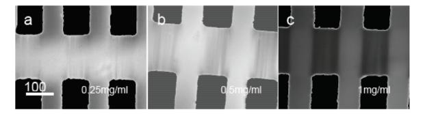
Figure 4.11 Optical images of CNT structures assembled on electrode arrays with the same configuration, under the same AC field, while with CNT suspension of different concentrations.
