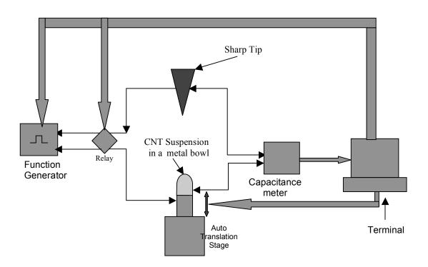
Figure 5.2 Schematic illustration of the automatic experimental setup used to fabricate CNT fibrils by dielectrophoresis.
