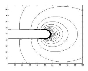
Figure 1.5 Compressed equipotential lines near the sharp protrusion of a metal surface (unit of x and y axis: nm, equipotential spacing: 10V) [45].
