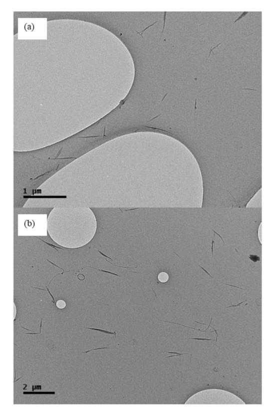
Figure 3.3 TEM pictures of shortened SWNT bundles to average length a. 0.5  $\mu$ m and b. 1.5  $\mu$ m. The tubular structure was not damaged during the chemical etching.
