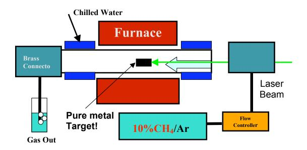
Figure 2.3 Same setup described in Figure 2.1, a cylinder of methane / Ar mixture is used instead of pure Ar gas and a pure metal target is used.
