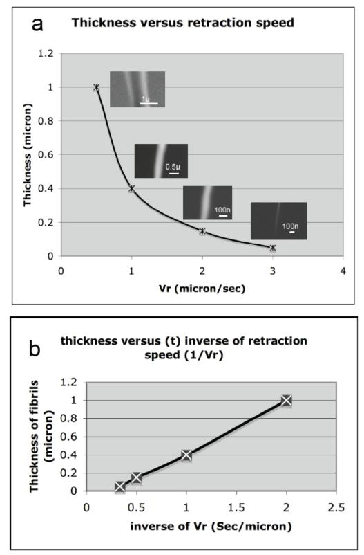
Figure 5.9 Fibril thickness plotted again retraction speed (a) and inverse of retraction speed. (b)
