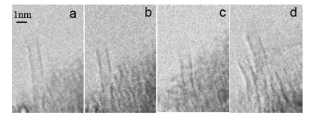
Figure 3.5 HRTEM images of individual SWNTs after oxidation and vacuum annealing at 400 °C for 10hrs. The results show that the ends of the SWNTs stayed open after the 400 °C annealing. (The scale bar is the same for all 4 images)
