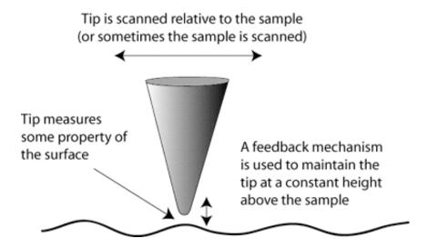
Figure 1.4 Schematics drawing to illustrate the working mechanism of a SPM probe [32]
