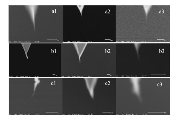
Figure 5.10 SEM images of CNT fibrils grown on commercial AFM probes. (a) AC field of 2 V was applied; (b) AC field of 5 V was applied; (c) AC field of 10 V was applied. The same CNT suspension was used and the probe was retracted from the suspension at maximum speed right after it reached the suspension.
