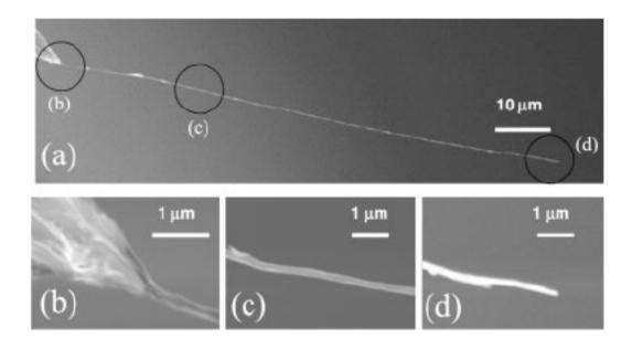
Figure 4.13 SEM images of CNT fibril assembled on the apex of an etched tungsten probe. (a) overall morphology; (b) The interface between the fibril and the W probe; (c) A mid segment of the fibril; (d) The end of the fibril. The concentration of the suspension used was 0.01mg/ml. [22]
