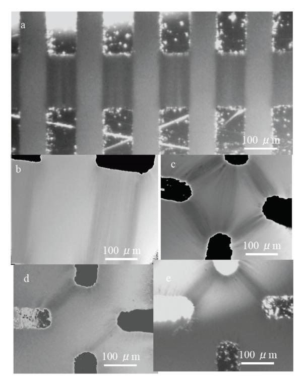
Figure 4.7 Different CNT structures fabricated by using different electrode array configurations. (a), (b) protruded electrodes with flat front facing each other, CNT structures were found to form exactly between the facing electrodes and CNT bundles within the structure are parallel to the electrical field; (c),(d),(e) Same set of electrode array, while when different electrical connection were used, different CNT structures can be fabricated.
