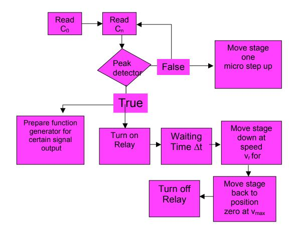
Figure 5.5 Flow chart of the Lab View program, by which the automation of the fabrication process is realized.
