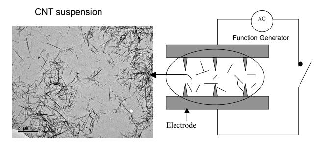
Figure 4.3 Illustration of Manipulation of CNTs on a patterned gold electrode array by dielectrophoresis. Left side is a TEM image of the CNT suspension used in this study.
