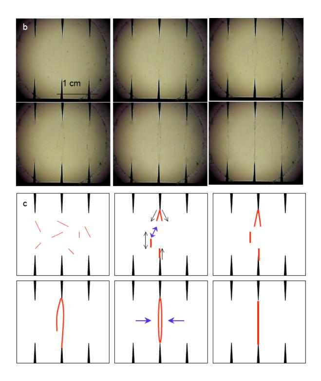
Figure 4.5 (a) Simulation of assembly process of CNTs between to facing protruded electrodes; (b) shows several frames from a recorded movie revealing the CNTs at different stages of the assembly process under AC field. In (c) a schematic is drawn according to the optical images.
