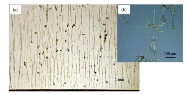
Figure 4.4 CNT structures formed between two planar electrodes. 25 V/mm of AC field was applied. (a) In situ optical image; (b) polarized light optical images of fibrils picked from the substrate.
