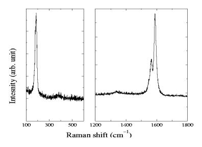
Figure 3.6 Raman spectroscopy data from chemically oxidized SWNTs indicates unchanged frequency of the characteristic RBM mode.
