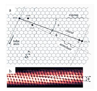
Figure 1.2 Structure of a SWNT related with its chiral vector. (a)A chiral vector  $C_h = n a_1 + m a_2$  is defined on the honeycomb lattice of carbon atoms by unit vector  $a_1$  and  $a_2$  and the chiral angle  $\theta$  with respect to the zigzag axis [5], (b) A high resolution scanning tunneling microscopy (STM) image showing the lattice structure of a chiral SWNT. The helical structure is clearly revealed [6].
