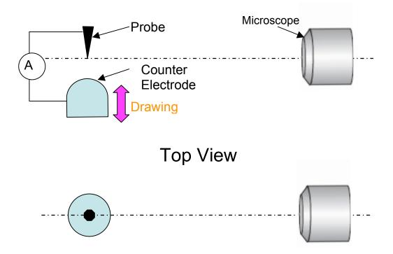
Figure 5.1 Schematics of the manual experimental setup for fabrication of CNT fibrils by dielectrophoresis.
