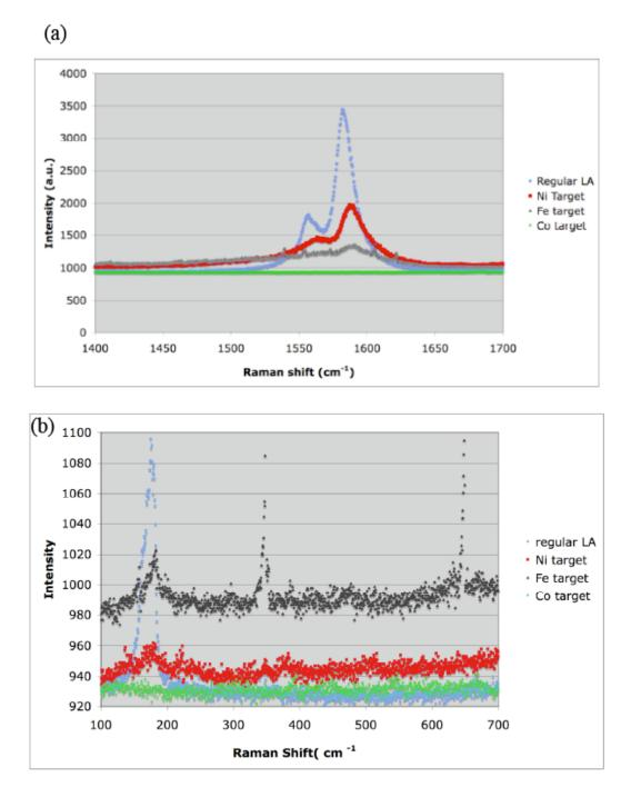
Figure 2.6 Raman spectral of SWNT synthesized by laser ablation method and laser CVD method by using Fe, Ni and Co pure metal rod targets. (a) high wave number G band sigal. (b) Low wave number breathing mode signal.
