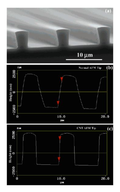
Figure 4.15 (a) Cross-sectional SEM image of a photoresist with 4.5-µm-deep trenches used to test the CNT AFM probe. (b and c) Height profiles measured from the same sample by a conventional Si AFM probe and the CNT probe, respectively. As shown, a nearly vertical sidewall (87°) was mapped by the CNT probe but not by the conventional AFM probe. The CNT probe remained intact after the measurement. [23]
