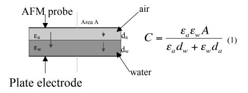
Figure 5.4 A model used to study the change in capacitance of the system. Where  $\varepsilon_a$  is the permittivity of air and  $\varepsilon_w$  that of water;  $d_a$  is distant from probe end to the surface of the suspension and  $d_w$  is depth of the suspension.
