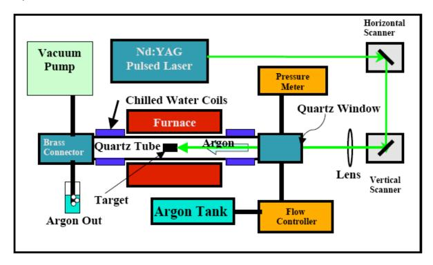
Figure 2.1 Laser ablation system for the synthesis of single wall nanotubebs. The focused laser beam scanned over the target surface using an XY raster. The formed nanotubes were carried by Ar and collected in a chill water cooled zone of the quartz tube.
