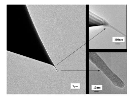
Figure 4.14 SEM images of CNT fibrils attached to commercial AFM probes by dielectrophoresis process. The SWNT bundle has a diameter of 20 nm near the tip and has conical geometry. [23]
