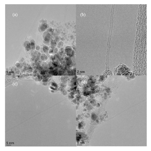
Figure 2.5 HRTEM images of as SWNT synthesized by laser CVD method. (a) iron targe (99.99% purity from Alfar Asear) was used; (b) Co targe (99.99% purity from Alfar Asear) was used; (c) and (d) Ni target (99.99% purity from Alfar Asear) was used. In all the experiments 10% methane was added to the flowing Ar, while flow rate was 400 sccm
