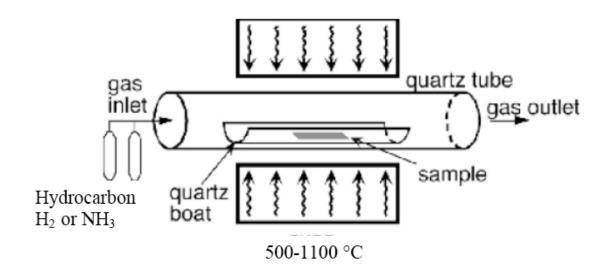
Figure 2.2 Supported catalysts CVD system, catalyst is deposited on a substrate, which is put into a heated up furnace, hydrocarbon is flowed into the furnace. [24]
