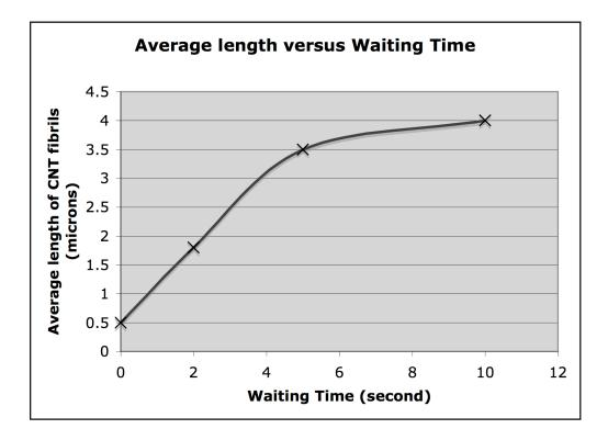
Figure 5.7 Average lengths of CNT fibrils plotted against waiting time. The average lengths were proportional to  $\Delta t$  when  $\Delta t$  is shorter than 5 second, then the average length changes little when  $\Delta t$  was further increased.
