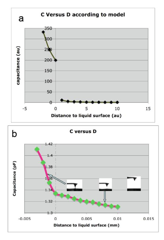
Figure 5.5 Change in system capacitance while the probes move towards the suspension. (a) Capacitance versus distance curved predicted by the model in figure 5.4; (b) Capacitance versus distance curves measured in experiment.
