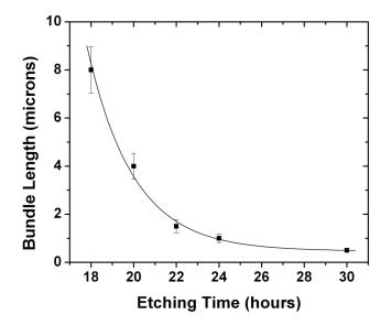
Figure 3.2 Experimenatly observed relationship between the average bundle length and the processing time. This relationship was determined for SWNTs produced by laser ablation process [11].
