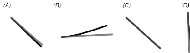
Figure 3.16. Plots of the configuration of a rigid wing (gray line) and a flexible wing (black line) engaged in the vertical stroke at Re=10 , shown at (A) the beginning of downstroke, (B) midway through downstroke, (C) at the beginning of upstroke, and (D) midway through upstroke. The greatest deformation among all of the strokes analyzed occurs during the middle of downstroke for the vertical stroke.
