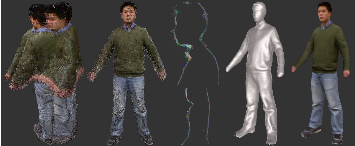
(a) Pre-aligned Point Clouds (b) Post-aligned Point Clouds (c) Cross Section of alignment (d) Fused Scan (e) Fused Scan with Color
