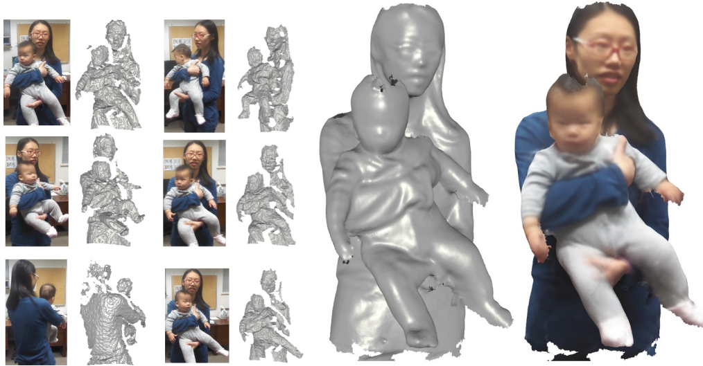
Figure 5.1: A mother holds an energetic baby while rotating in front of a Kinect camera. Our system registers scans with large deformations into a unified surface model.
