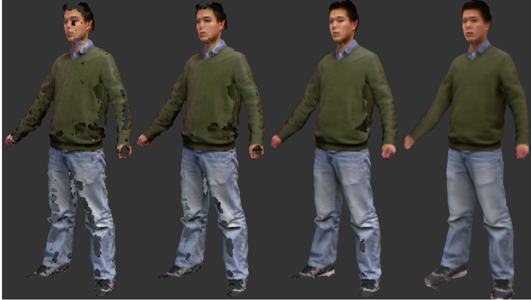
Figure 1.4: Data accumulation for a person turning around in front of depth sensors. Surfaces after fusing 1, 5, 50, and 150 frames of data.
