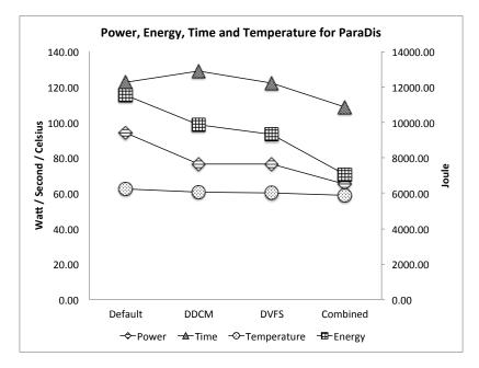
Figure 4.5: Execution metrics for ParaDis while using ACR with DDCM, DVFS and both on 32 nodes (1024 cores). Note that the values are discrete with links only serving as visual cues.
