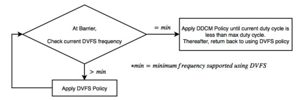
Figure 4.2: Working of the Combined policy that uses both per-core DVFS and DDCM
