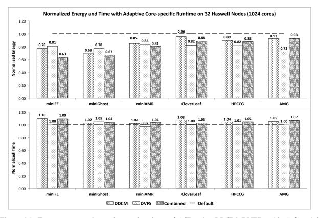
Figure 4.4: Energy consumption and execution times of ACR using DDCM, DVFS and both for mini applications
