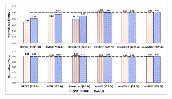
Figure 5.5: Energy consumption and execution times using coarse (CDP) and fine-grained (FDP) dynamic policy for mini applications
