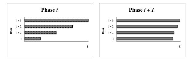
Figure 3.1: (left) Each MPI process in an MPI application is observed to complete its phase i in a fraction of the time in which all processes reach the barrier at the end of phase i. The runtime uses this fraction to adjust the duty cycle for each process in phase i + 1, according to eqns (1) and (2). (right) If the work per process is similar in phase i + 1, the completion times will be more nearly equal, energy will be saved and perhaps time will be decreased.
