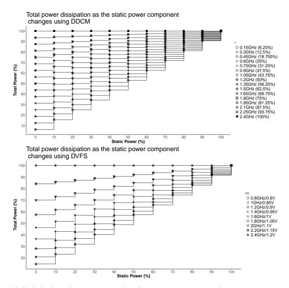
Figure 2.3: Variation in total power consumption of a processor core as the static power component changes while using DDCM and DVFS
