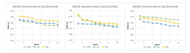
Figure 3.9: Execution times for ADCIRC with combinations of power cap and minimum threshold duty cycle
