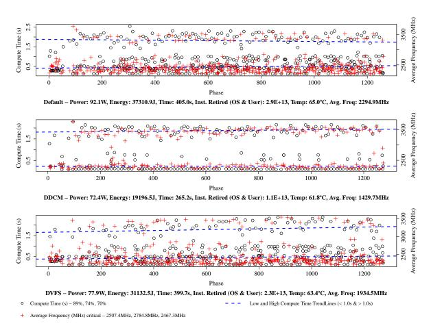
Figure 4.7: Critical Path Behavior for ParaDis running on 24 nodes (768 cores).
