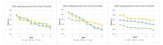
Figure 3.11: Execution times for LQCD with combinations of power cap and minimum threshold duty cycle
