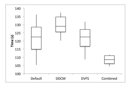
Figure 4.6: Variation in execution time of Paradis across all cores for 12 runs on 32 nodes
