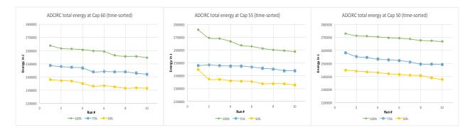
Figure 3.10: Energy consumed by ADCIRC with combinations of power cap and minimum threshold duty cycle
