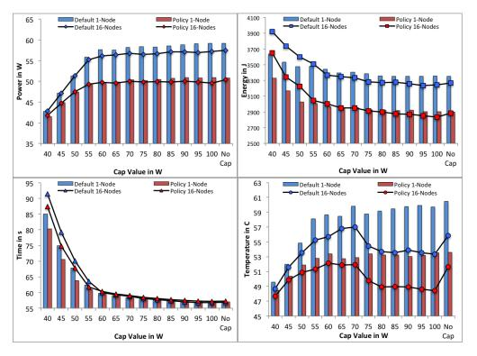
Figure 3.3: Power, Energy, Time and Temperature for Equally Shifting Load pattern
