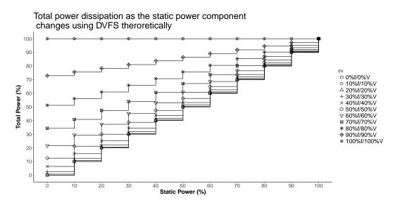
Figure 2.2: Variation in total power consumption of a processor core as the static power component changes while using DVFS theoretically
