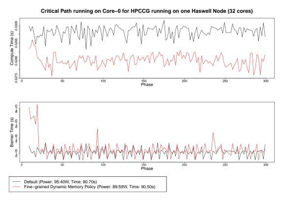
Figure 5.6: Compute and barrier times for HPCCG using fine-grained dynamic policy (FDP) on one Haswell node (32 cores). Power consumption and total execution time for default and FDP are also shown.
