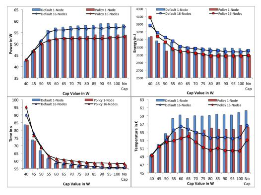
Figure 3.4: Power, Energy, Time and Temperature for Randomly Shifting Load pattern
