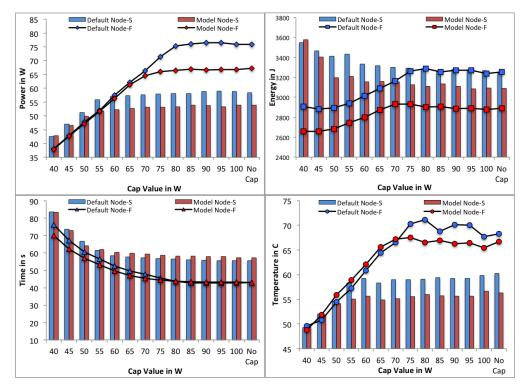
Figure 3.7: The graphs show variation in power, energy and time for two different nodes while using DDCM with RMR synthetic benchmark.
