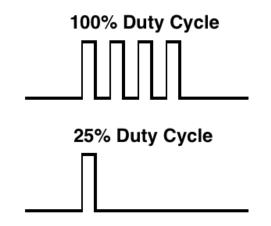
Figure 2.1: Dynamic Duty Cycle Modulation in operation
