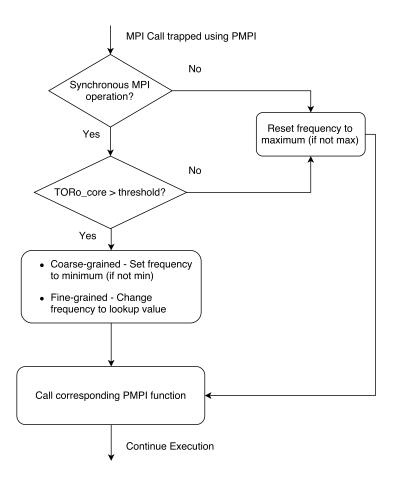
Figure 5.3: Flowchart of the dynamic policy using TORo\_core as the metric to throttle power using per-core DVFS
