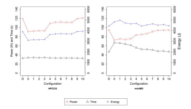
Figure 5.4: Effect of using different TORo\_core threshold values on HPCCG (memory constrained) and miniMD (compute bound) application energy and execution time within coarse-grained dynamic policy (CDP). Note that the values are discrete with links only serving as visual cues.
