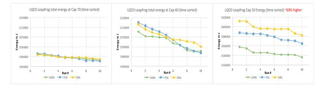
Figure 3.12: Energy consumed by LQCD with combinations of power cap and minimum threshold duty cycle
