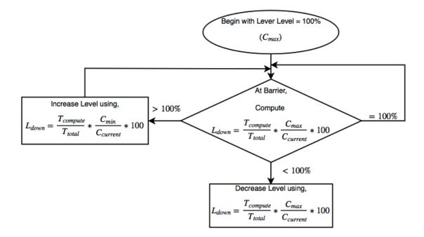
Figure 4.1: Working of the generic core-specific adaptive runtime policy
