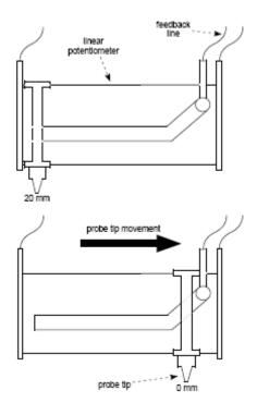
**Figure 2.3** Linear potentiometer system. Each probe tip slides on a linear potentiometer, which serves as both a linear slide and a linear position sensor.
