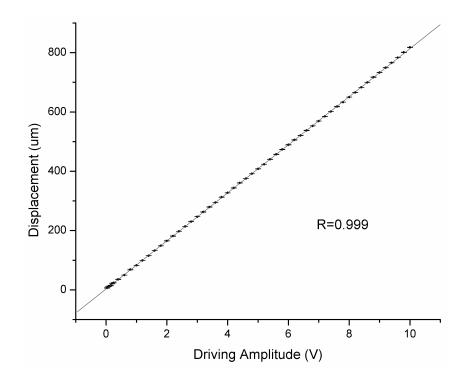
**Figure 7.2** Amplitude calibration and range of the CM-1. During system calibration, 25 Hz sinusoidal signals with variable peak-to-peak amplitude (driving voltage) were delivered by the NI DAQ analog output to the VCA coil of the CM-1. In this graph, the driving input voltage is plotted against the displacement (in  $\mu$ m) of the tip of the CM-1.
