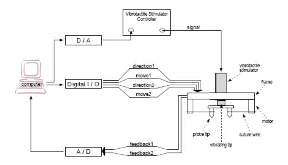
Figure 2.2 Block diagram of control system for the Two-Point Stimulator.
