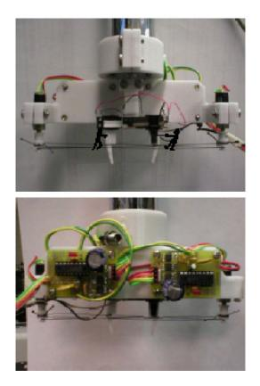
Figure 2.1 Images of the front and back of the Two-Point Stimulator as attached to a vibrotactile stimulator.
