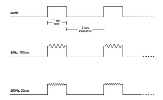
**Figure 3.2** Tracking protocol conditions. A tracking protocol was used to conduct a twopoint limen threshold test under three conditions of amplitude and frequency: static (no vibration), 25 Hz - 100  $\mu$ m, and 200 Hz - 20  $\mu$ m.
