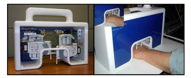
**Figure 7.1** Images of the Cortical Metrics (CM-1) stimulator. Left panel: Front view of the stimulator with a clear panel to allow visibility of internal components. Right panel: Probe tips detect the surface of the skin automatically (insert: close-up view).
