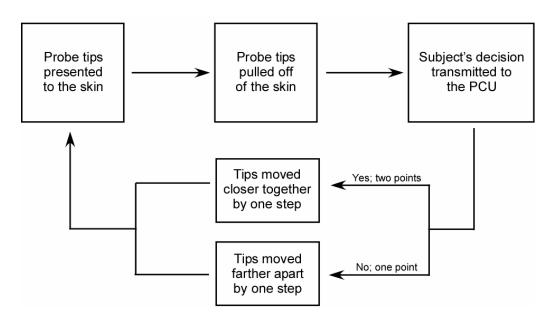
**Figure 3.1** Flowchart of the modified Bekesy tracking protocol used to determine the two-point limen of a subject with the Two-Point Stimulator.
