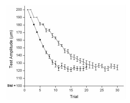
**Figure 7.4** Comparison of tracking paradigms. Subject performance is tracked with a 2 up / 1 down protocol (open square plot) and compared with a modified tracking protocol (closed circle plot; 1 up / 1 down tracking for the first 10 trials and 2 up / 1 down for the last 10 trials).
