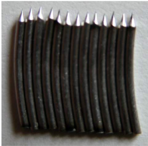
(a) A batch of uniformly bent pin with one sharpened tip.
