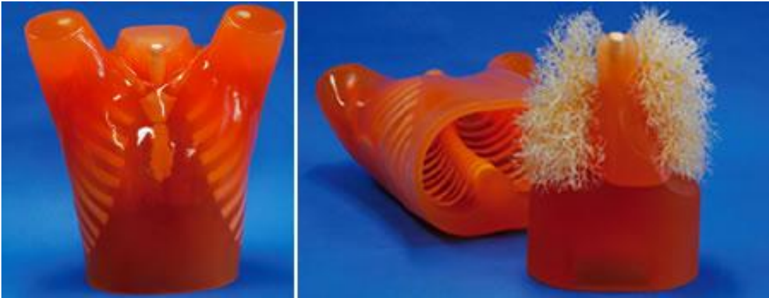
Figure 4.1: An anthropomorphic chest phantom (left) with realistic lung vessel structures (right).
