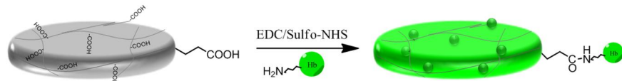
Figure 3.2 Scheme for the conjugation chemistry between carboxyls of particles and lysines of Hb.
