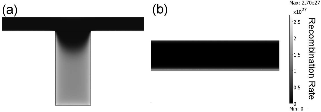
Figure 4.6: Bimolecular recombination rate, B_{photo} in units of (1/m^3s) , for (a) PC and (b) planar cells. Very low bimolecular recombination occurs in the flash layer of the PC cell and the entire planar cell. Due to the weak internal electric field in the nanostructured layer of the PC cell, strong recombination occurs.
